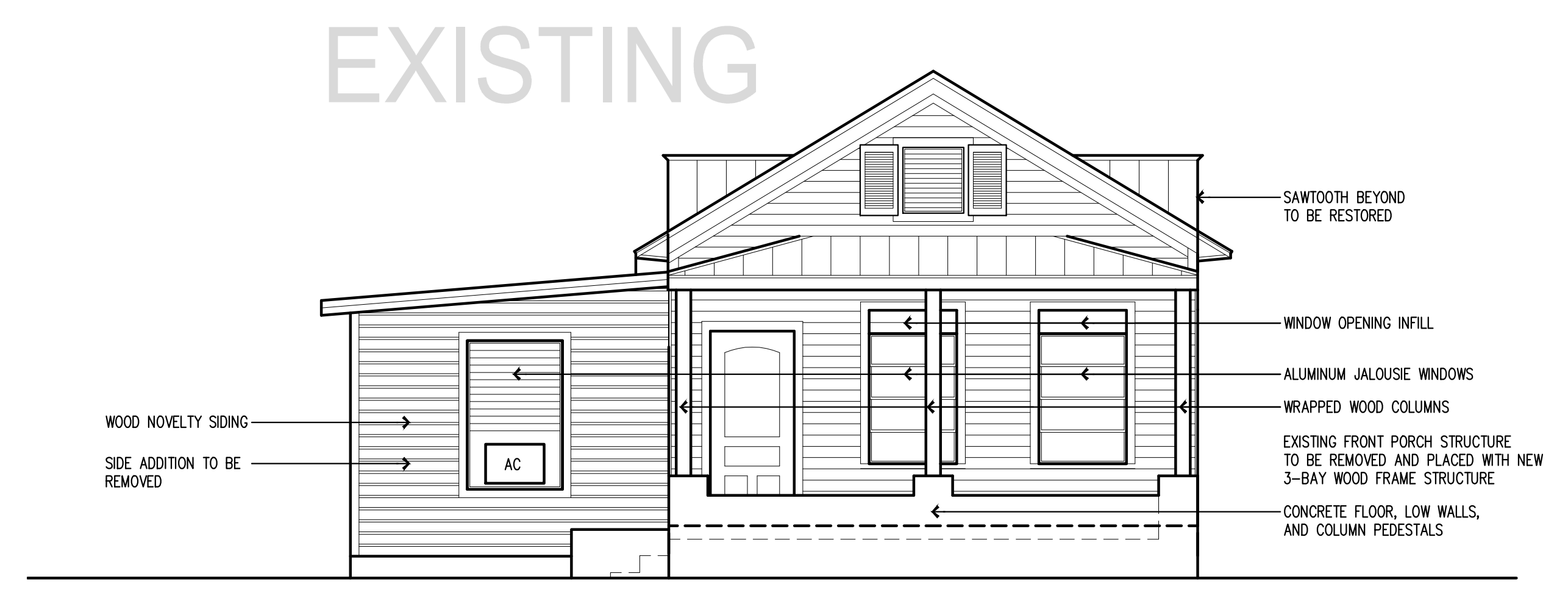
EXISTING FRONT ELEVATION 1/4"=1'-0"
