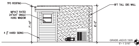
5 PROPOSED SIDE POOL HOUSE SCALE: 1/4"=1'-0"
