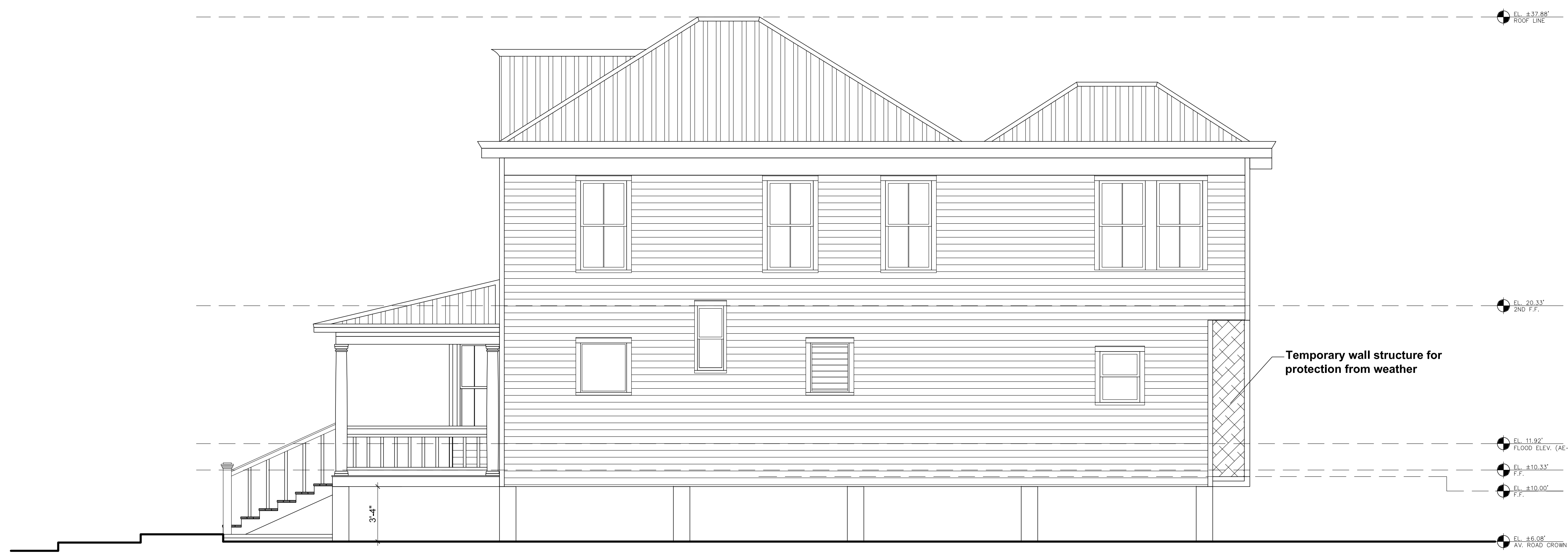
Weather Enclosure - Right Side Elevation SC. 1/4" = 1' - 0"
