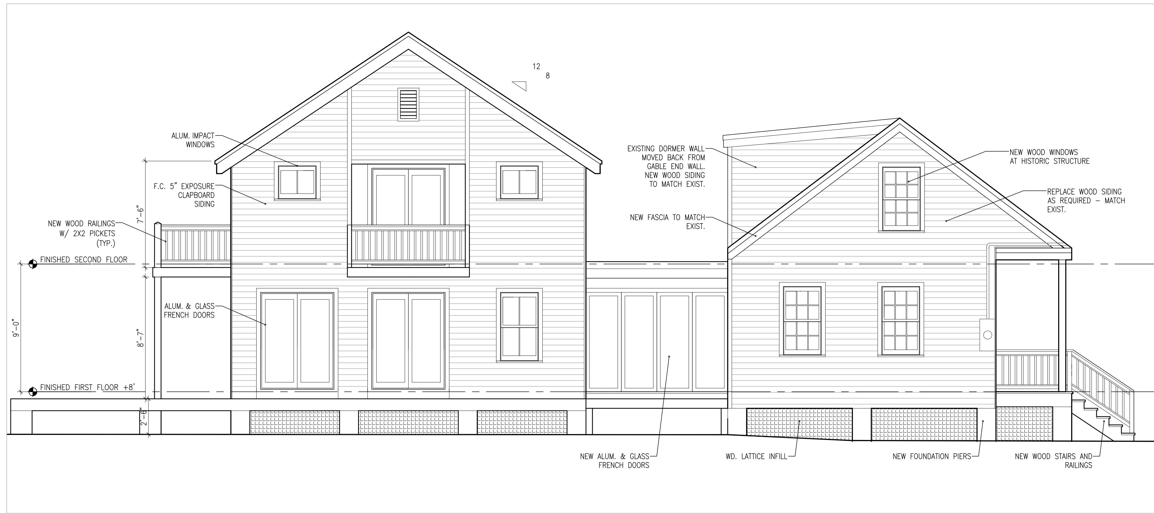
2 SIDE ELEVATION NORTH A31 SCALE: 1/4"=1'-0"
