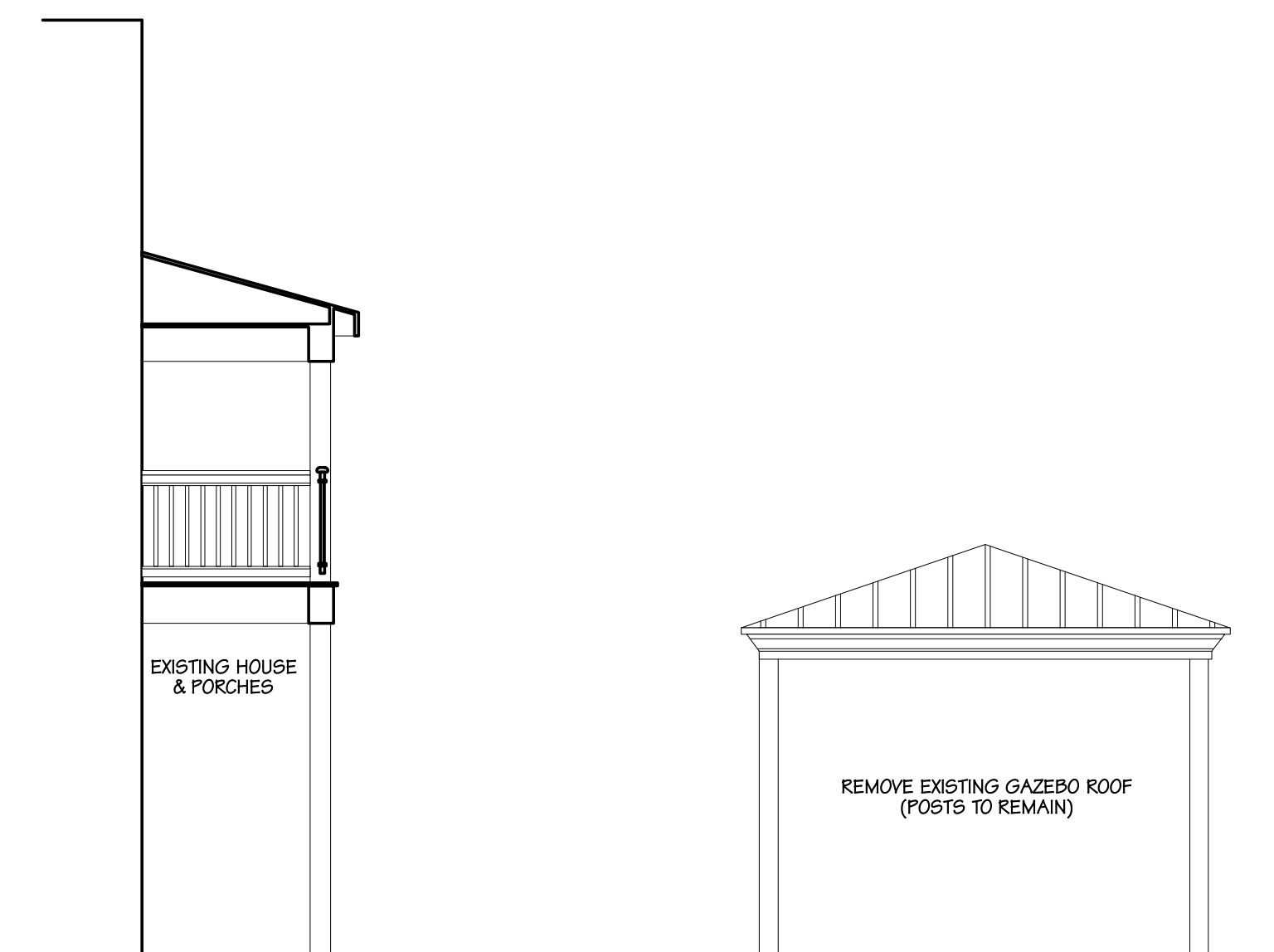
GAZEBO PROPOSED WEST ELEVATION scale: 1/4"=1'-0"
