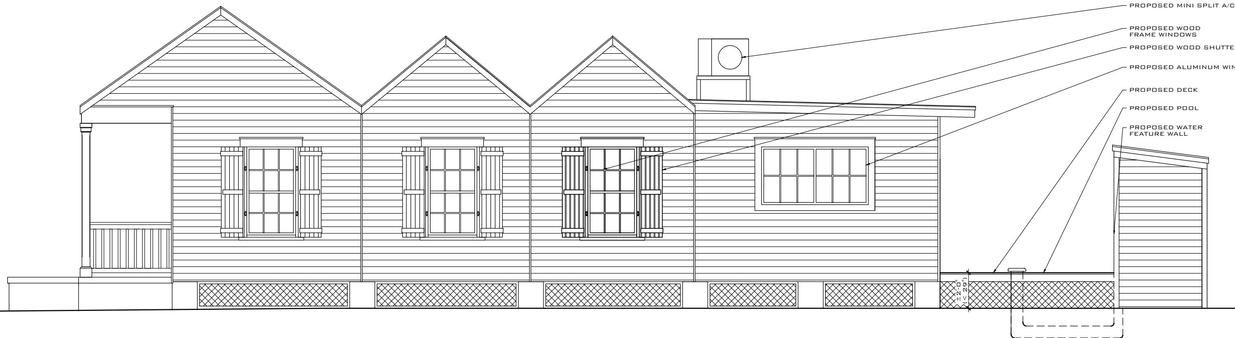
PROPOSED RIGHT ELEVATION SCALE: 3/16" = 1'-0"
