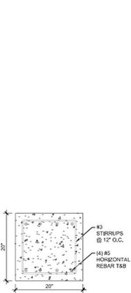
FOUNDATION PILE TO BE DESIGNED BY GEOTECHNICAL ENGINEER TO WITHSTAND ANY GRAVITY LOAD OF 40 TONS & LATERAL LOAD OF 4 TONS
