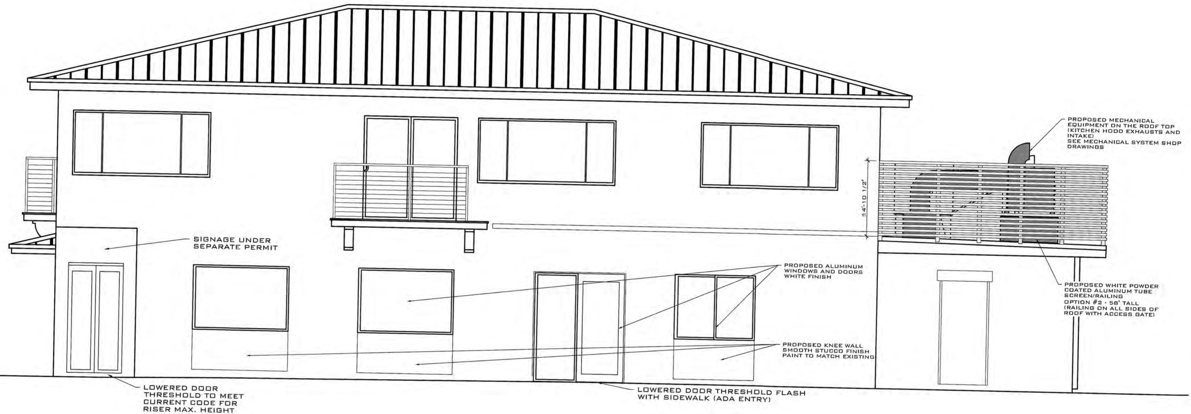
PROPOSED SIDE ELEVATION (CENTER ST) OPTION 2 - 4.9FT TALL SCREEN RAILING SCALE: 1/4" = 1'-0"
