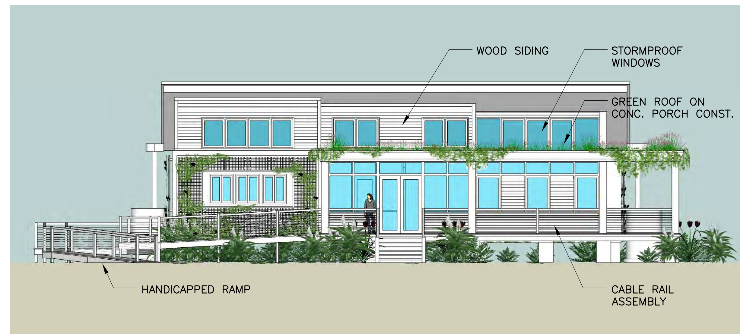
SOUTH ELEVATION - FRONT
