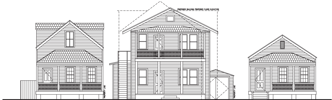
2 SITE ELEVATION ILLUSTRATING PREVIOUS STRUCTURE W/ PROPOSED BUILDING OVERLAY AT PROPOSED FLOOD ELEVATION. A3 / SCALE: 3/16" = 1'-0"
