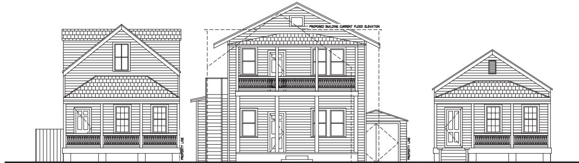
4 SITE ELEVATION ILLUSTRATING PREVIOUS STRUCTURE W/ PROPOSED BUILDING OVERLAY AT CURRENT FLOOD ELEVATION. A3 / SCALE: 3/16" = 1'-0"
