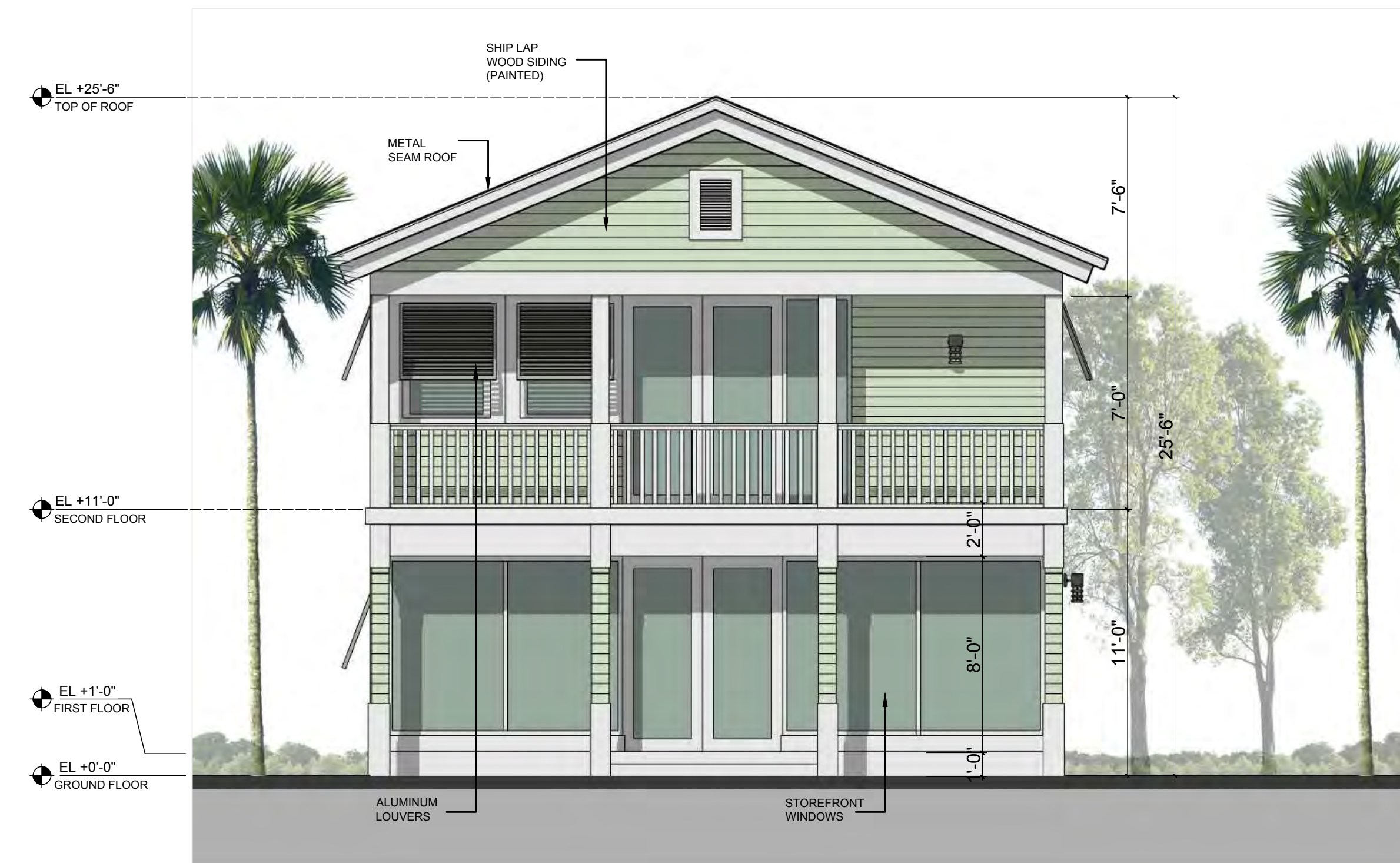
SOUTH-EAST ELEVATION (FRONT)
