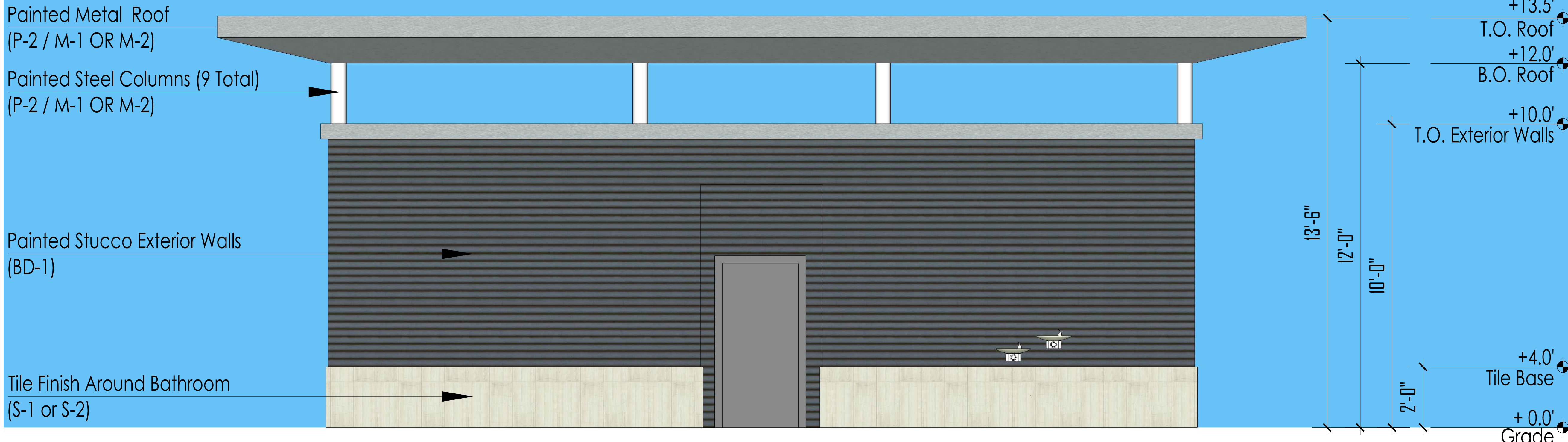
2 AMPHITHEATER BATHROOM - SOUTH ELEVATION
