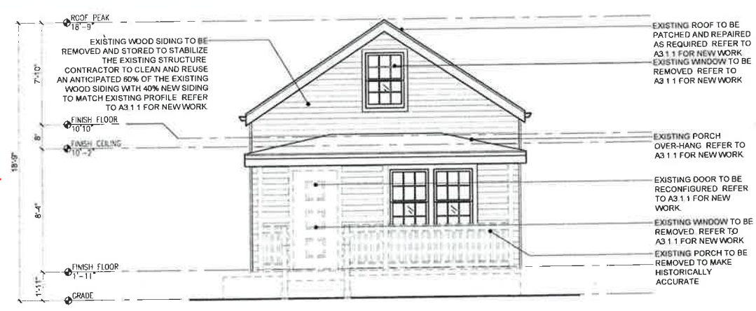
1 DEMOLITION SOUTH ELEVATION SCALE: 1/4"=1'-0"
