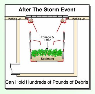
The coarse screen provides additional filtered flow with less chance for obstruction than either the medium or fine screen. The coarse screen is sized to capture floatables like foliage and litter. At this stage water is flowing through all the different sieve size screens, the turbulence deflector continues to dramatically reduce the turbulence in the lower filtration chamber, and sediment continues to settle and collect toward the bottom.
