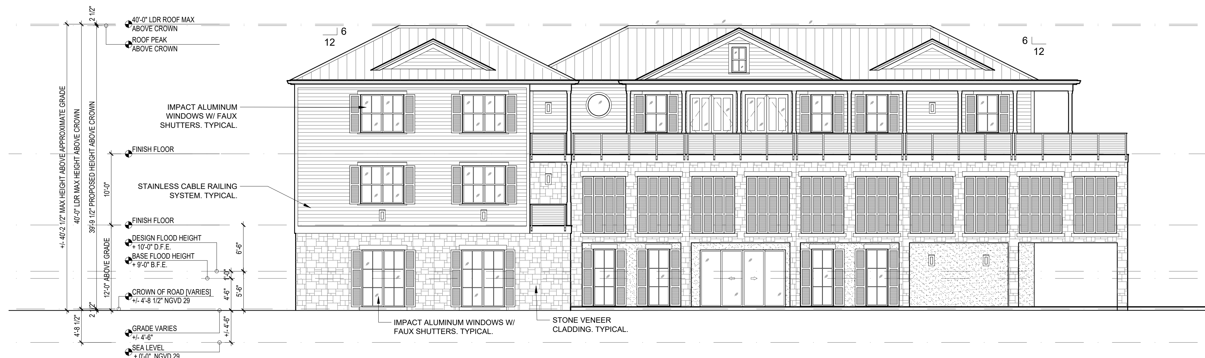
2 HOTEL LOBBY BUILDING: EAST ELEVATION [GULF] SCALE: 1/8"=1'-0"
