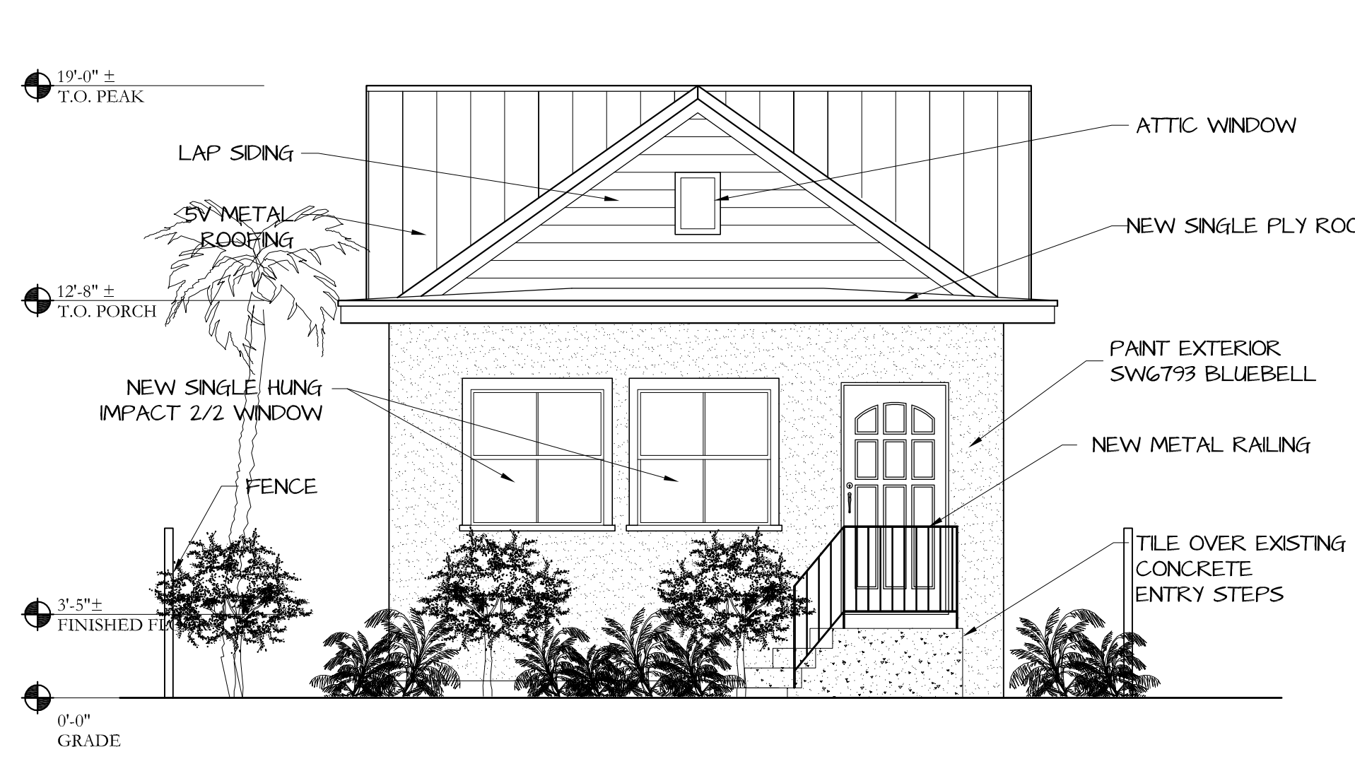
NORTH ELEVATION (PROPOSED) 1/4" = 1'-0"
