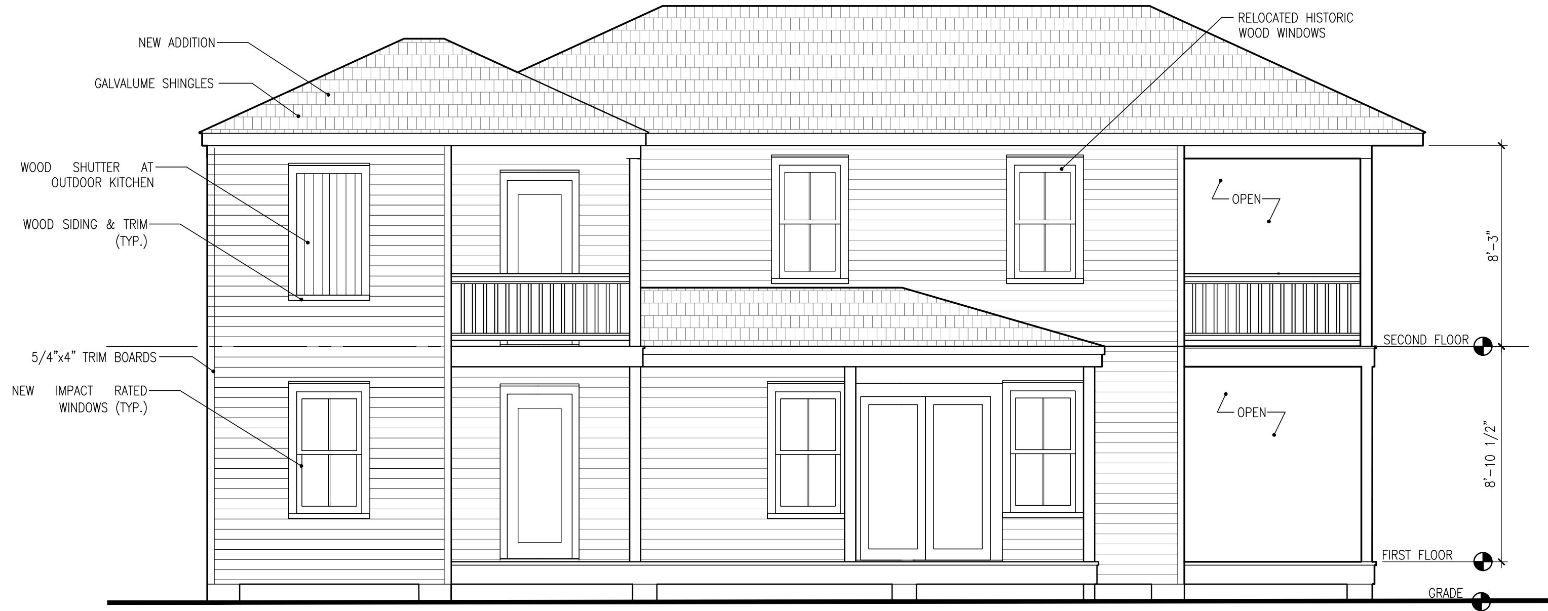
4 WEST ELEVATION A3.1 SCALE: 1/4"=1'-0"
