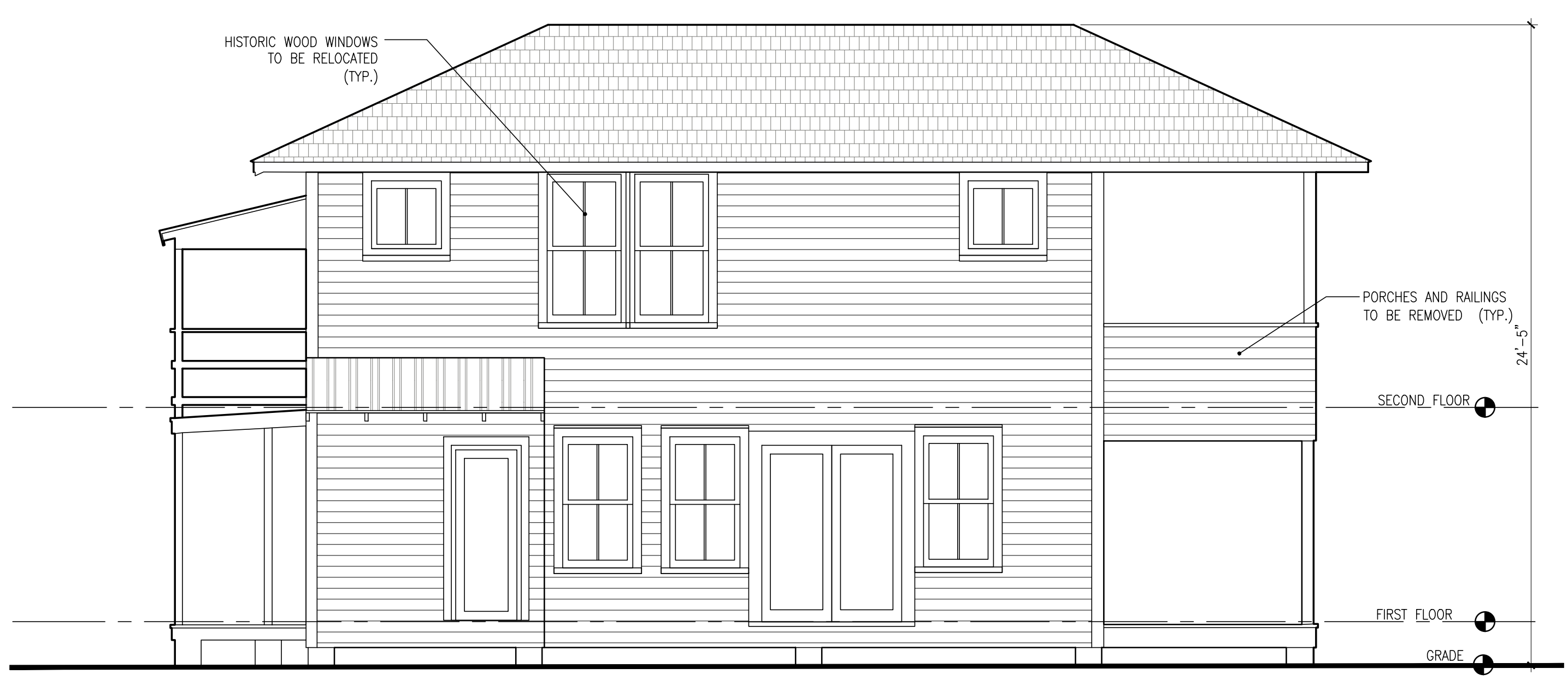
4 WEST ELEVATION SCALE: 1/4"=1'-0"
