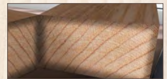
Traditional treatments only protect the outer surface
