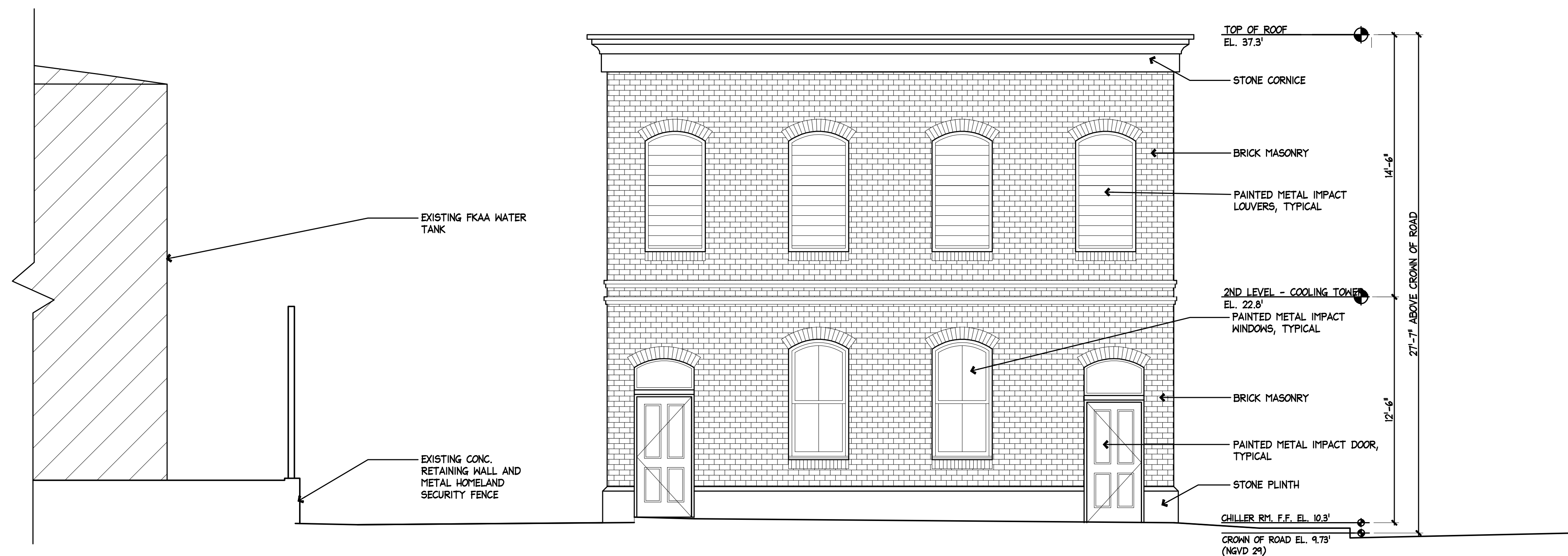
1 M2.4 PROPOSED NORTH EXTERIOR ELEVATION SCALE: 1/4"=1'-0"
