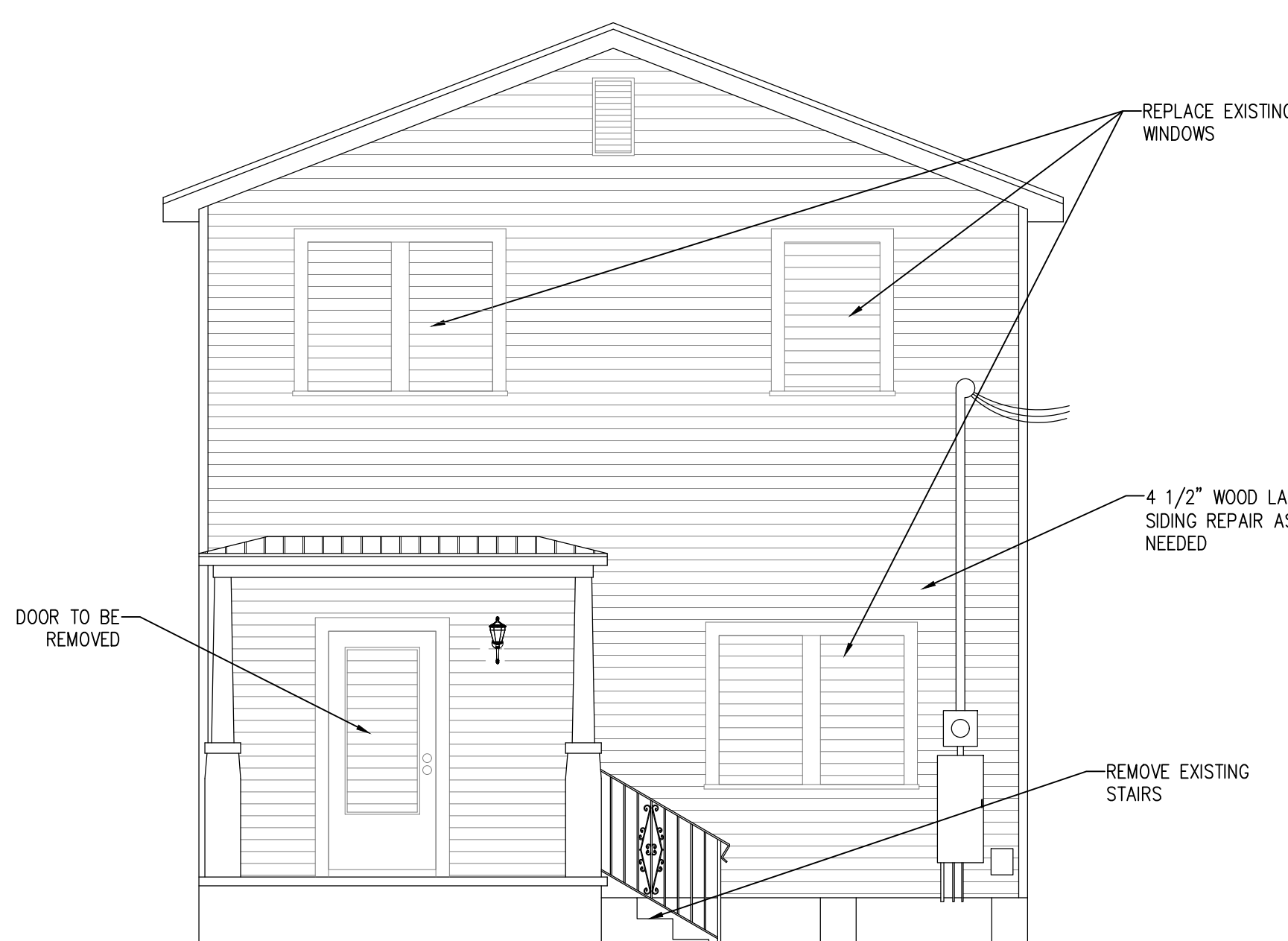
(PRE CONSTRUCTION) EXISTING FRONT ELEVATION
