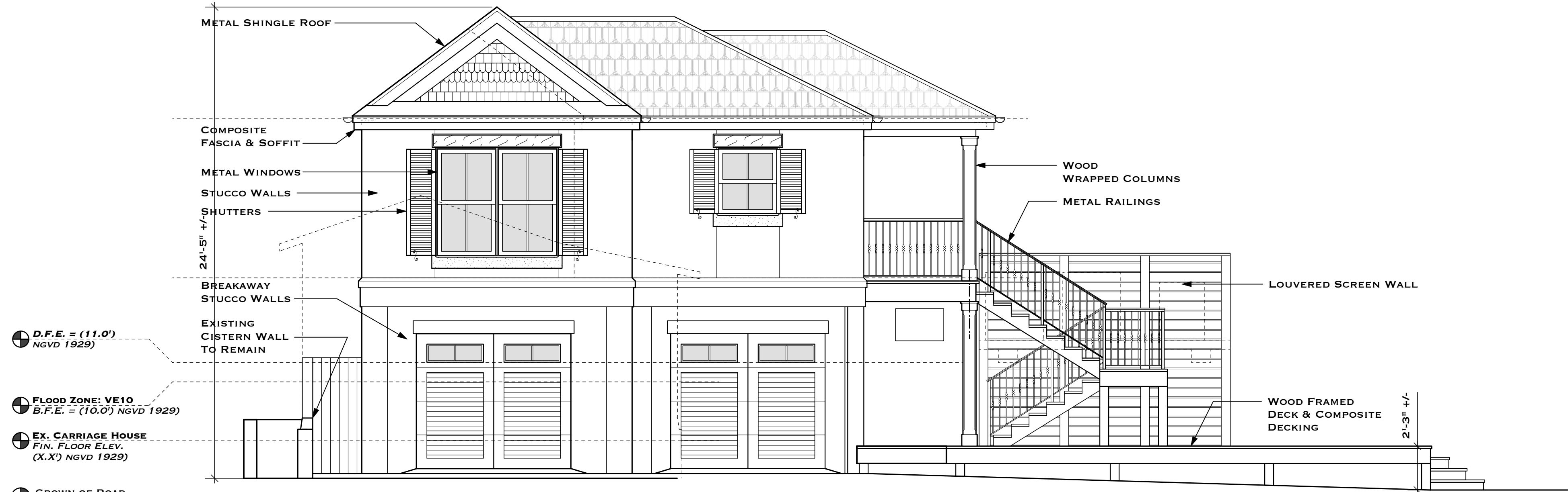
1 WHITEHEAD STREET GARAGE ELEVATION A3.3 SCALE: 1/4" = 1'-0"
