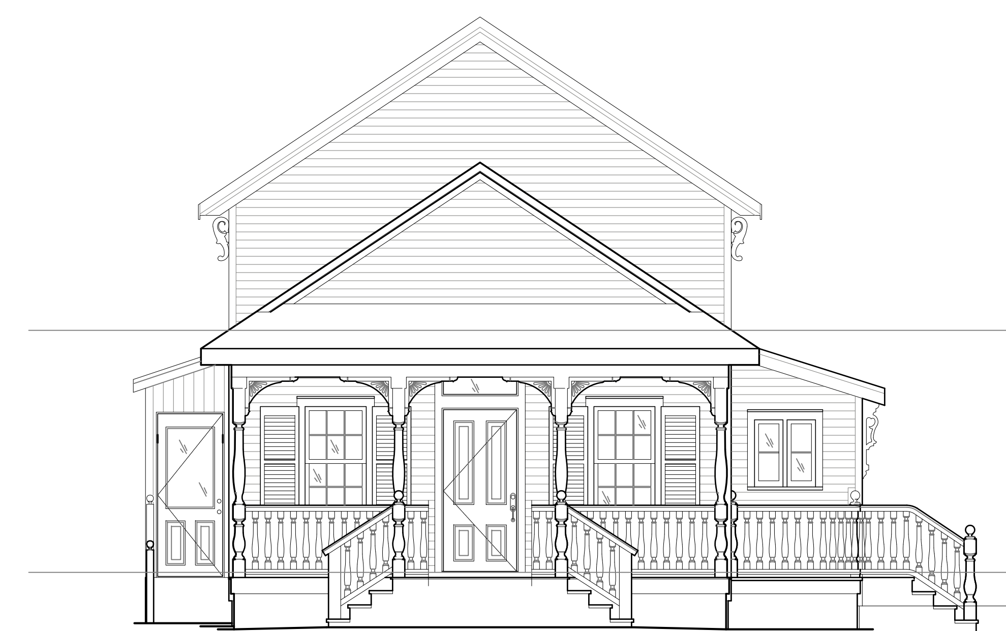
1 EXISTING WEST ELEVATION AE3.1 SCALE: 1/4"=1'-0"
