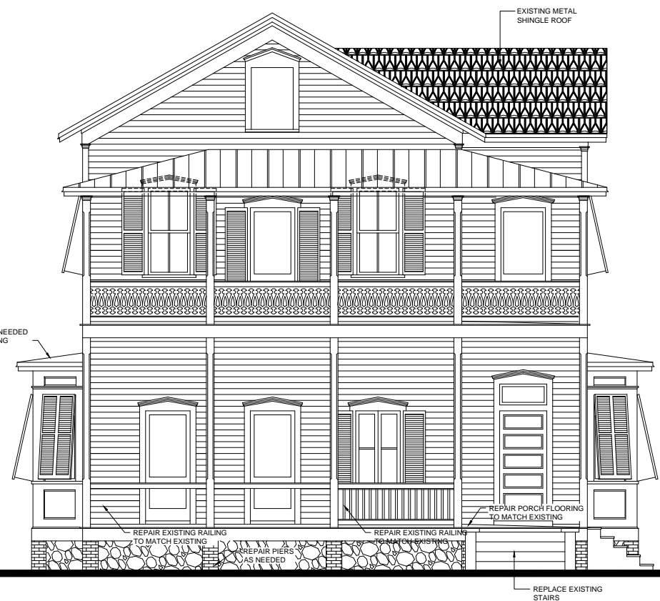
EXISTING NORTHEAST ELEVATION
