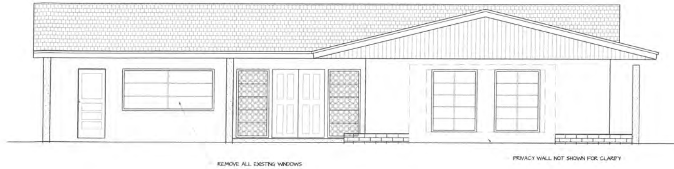
SOUTH ELEVATION (EXISTING) 1/4" = 1'-0"
