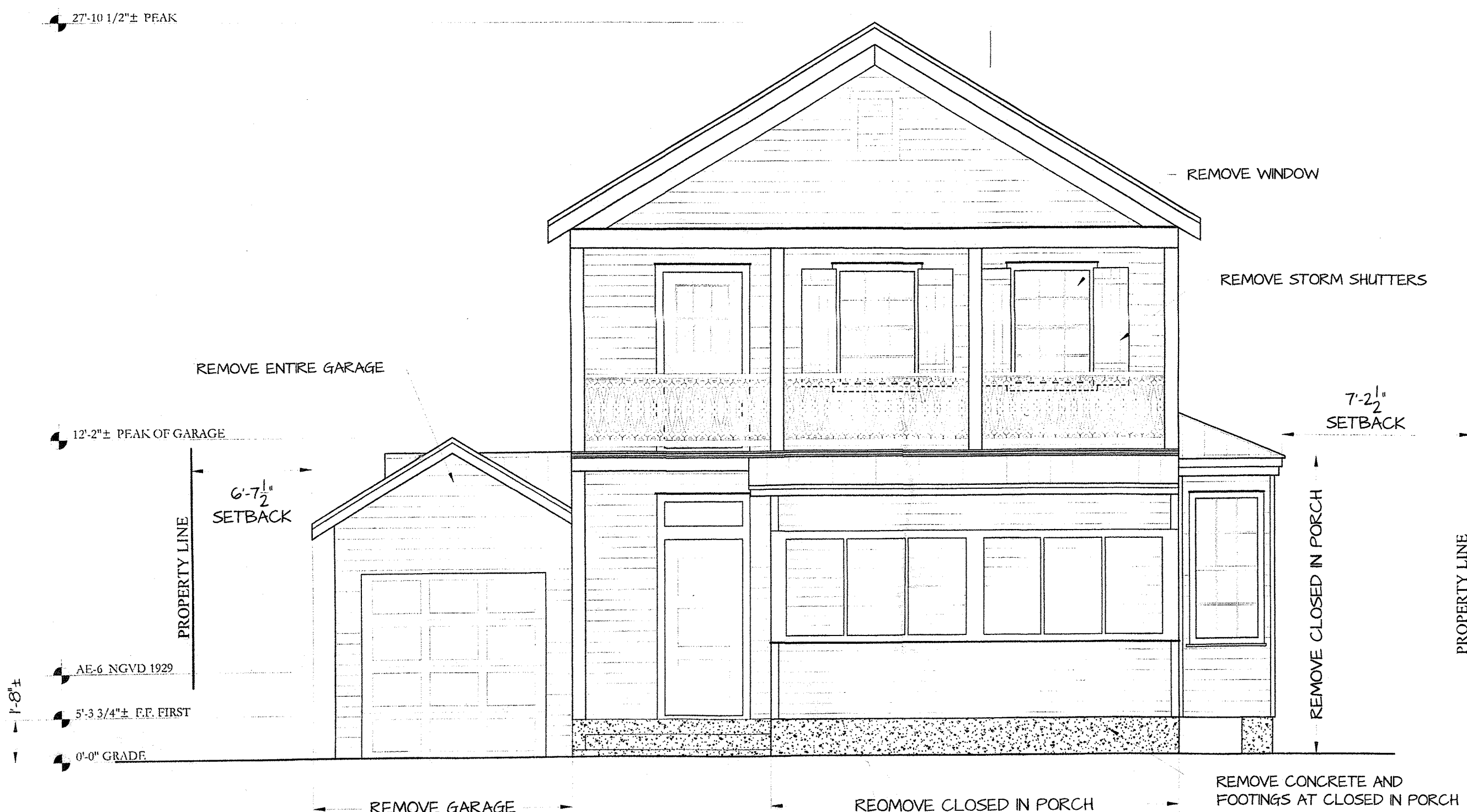
SOUTH ELEVATION (EXISTING/ DEMO) 1/4" = 1'-0"
