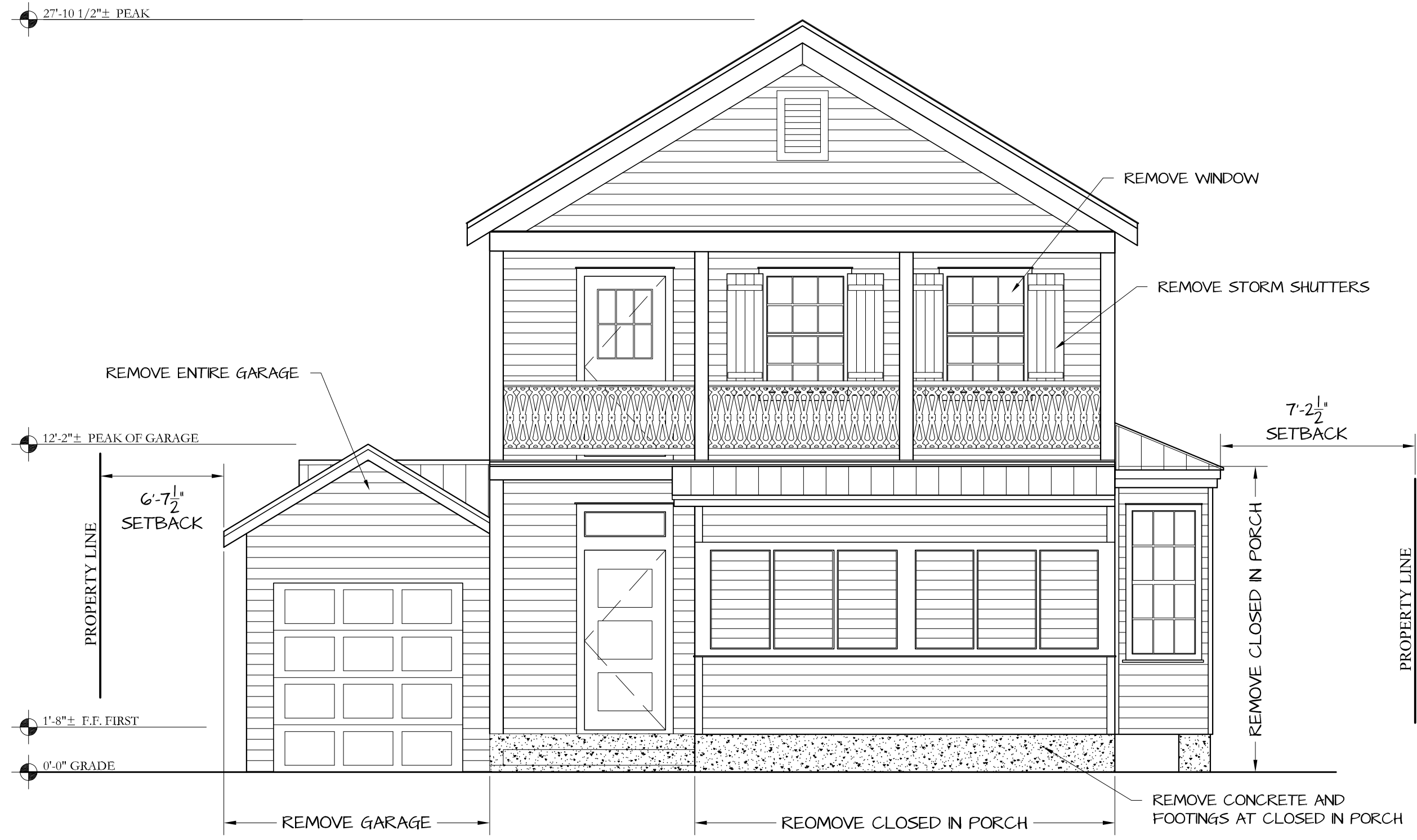
SOUTH ELEVATION (EXISTING/ DEMO) 1/4" = 1'-0"
