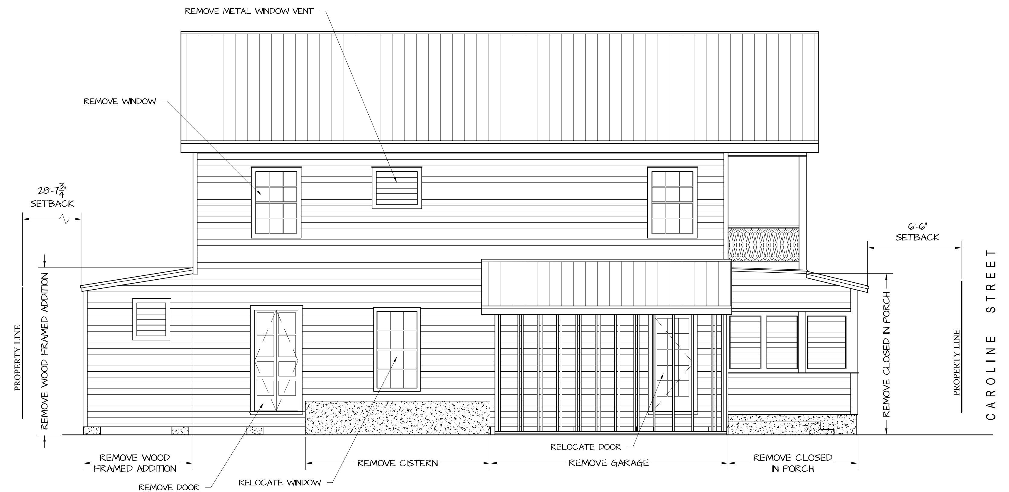
WEST ELEVATION (EXISTING/ DEMO) 1/4" = 1'-0"
