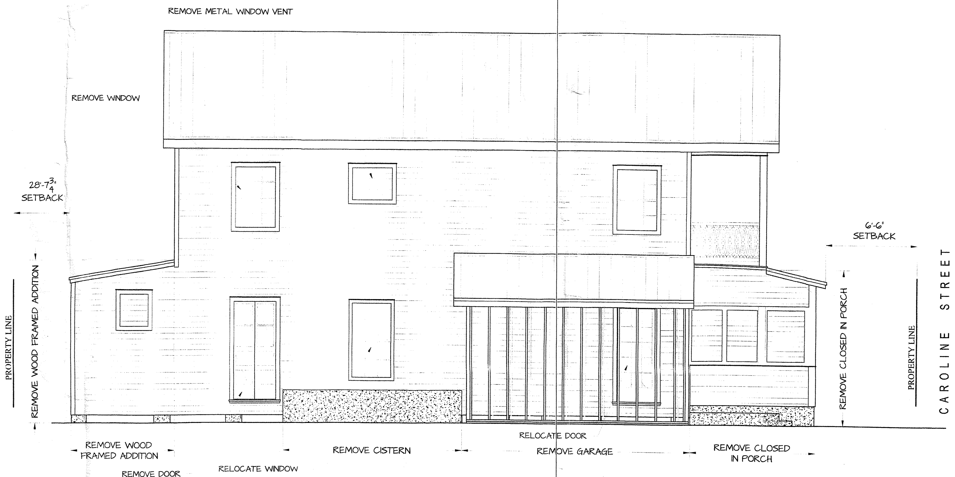
WEST ELEVATION (EXISTING/ DEMO) 1/4" = 1'-0"
