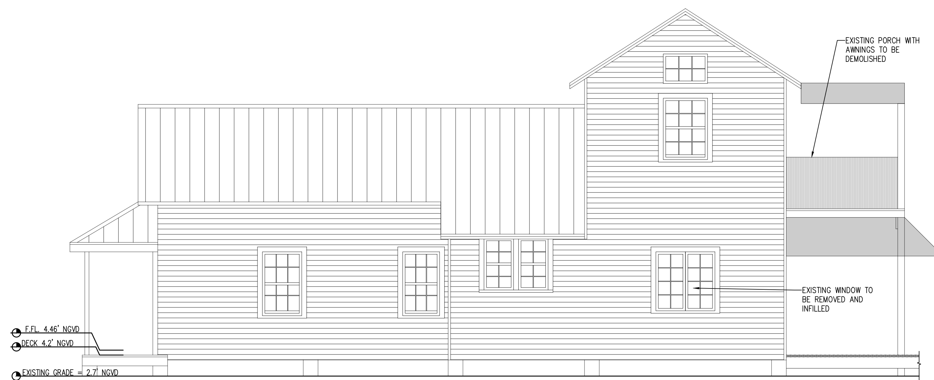
EXISTING SIDE ELEVATION
