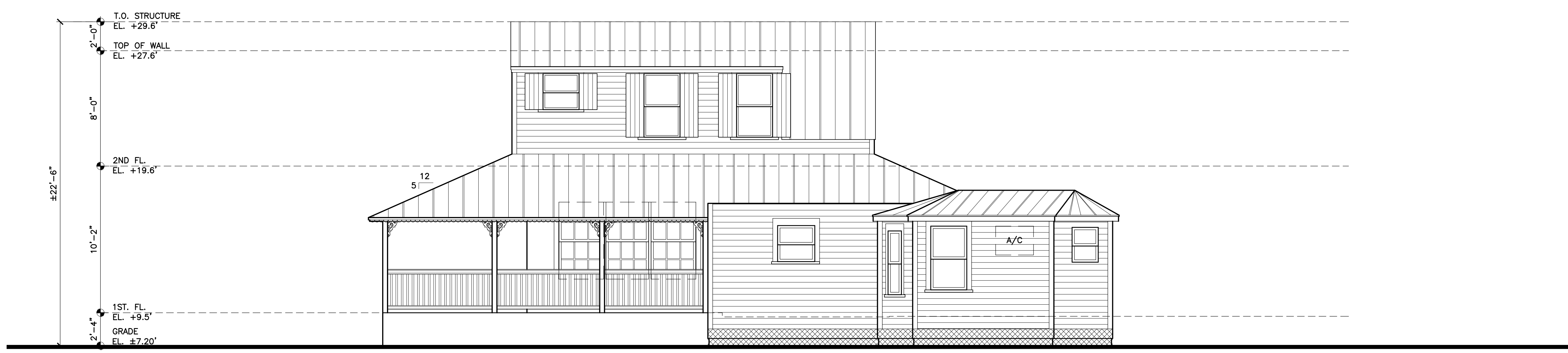
1 EXISTING HISTORIC BLDG SIDE ELEVATION
