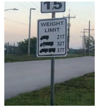
Exhibit 5-2. Weight Limit Sign on Bridge to Fleming Channel
