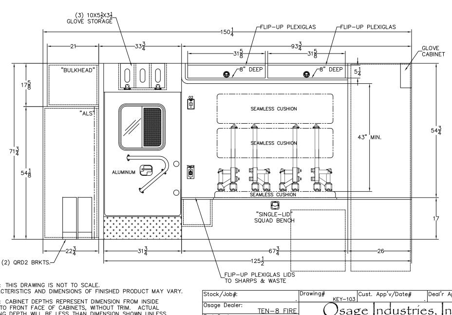
NOTES: CABINET DEPTHS REPRESENT DIMENSION FROM INSIDE REAR TO FRONT FACE OF CABINETS, WITHOUT TRIM. ACTUAL WORKING DEPTH WILL BE LESS THAN DIMENSION SHOWN UNLESS OTHERWISE SPECIFIED.
