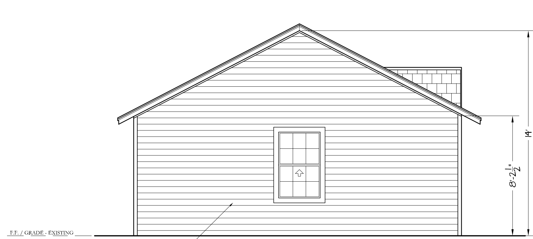
WEST ELEVATION (EXISTING) 1/4" = 1'-0"
