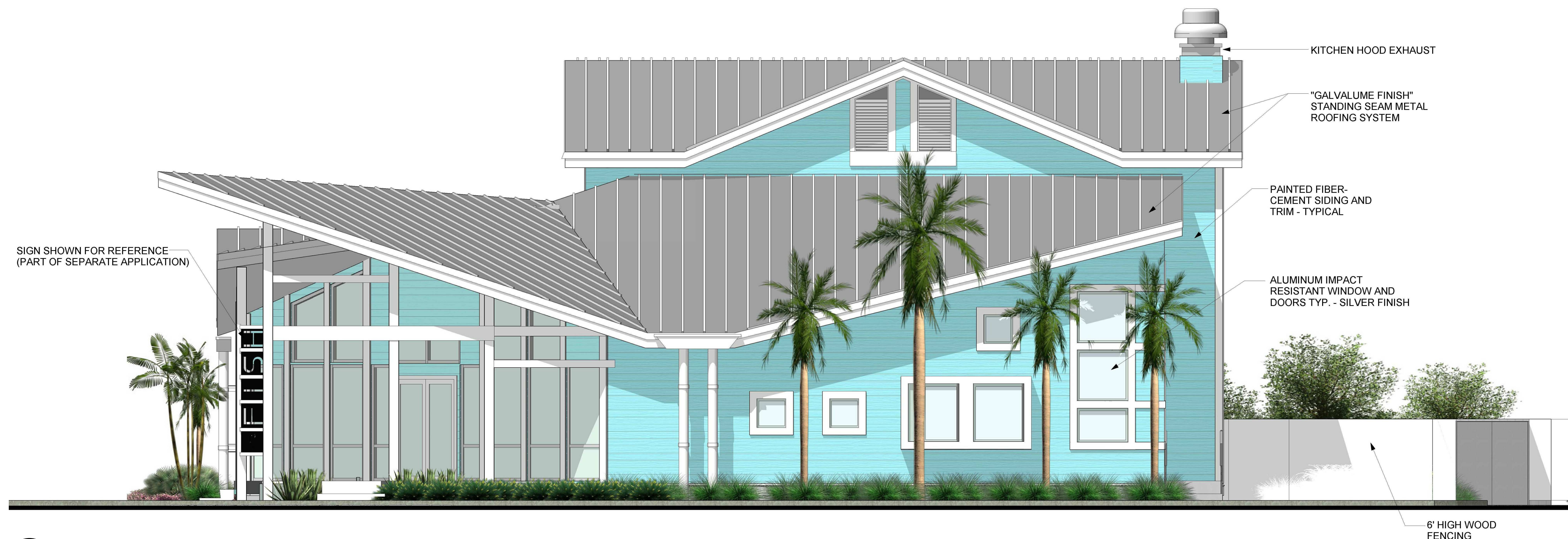
1 A-5 PACKER STREET ELEVATION SCALE 1/4" = 1'-0"
