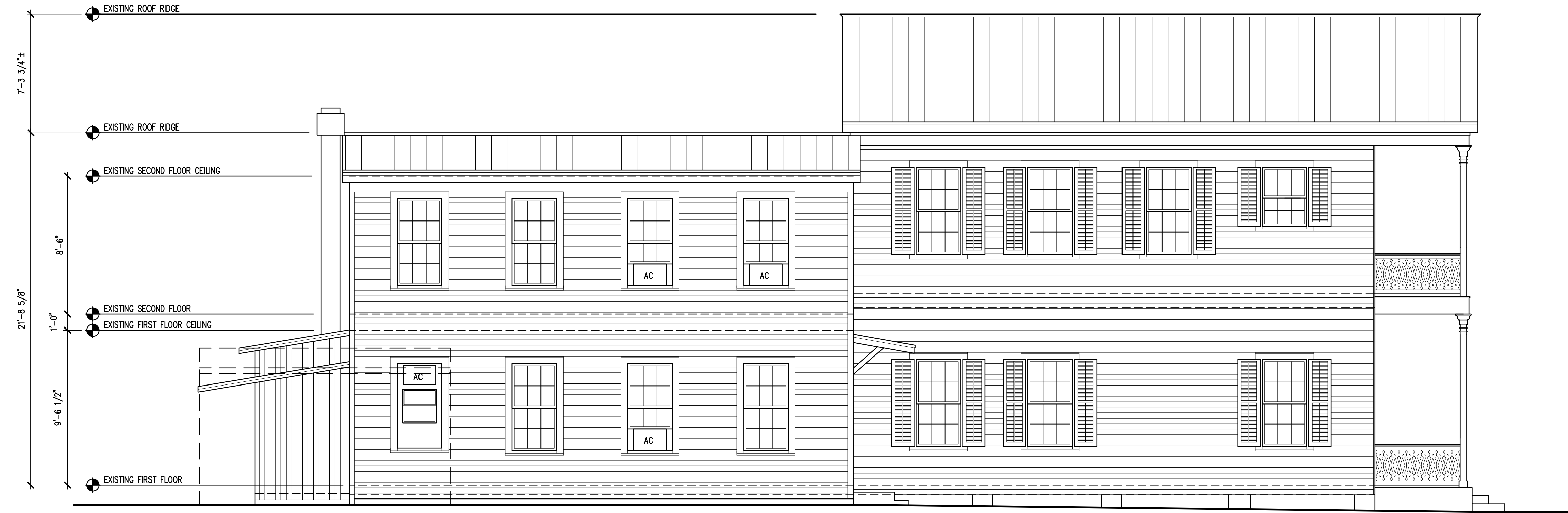
EXISTING WEST SIDE ELEVATION 1/4"=1'-0"
