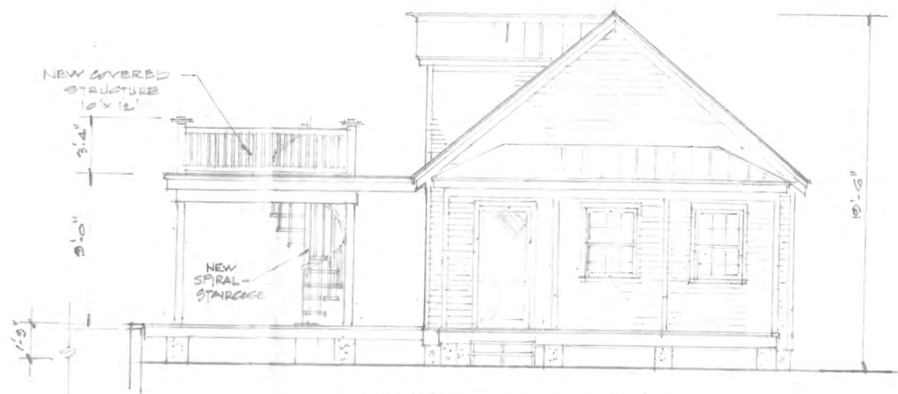
NORTH ELEVATION SCALE 3/16"
