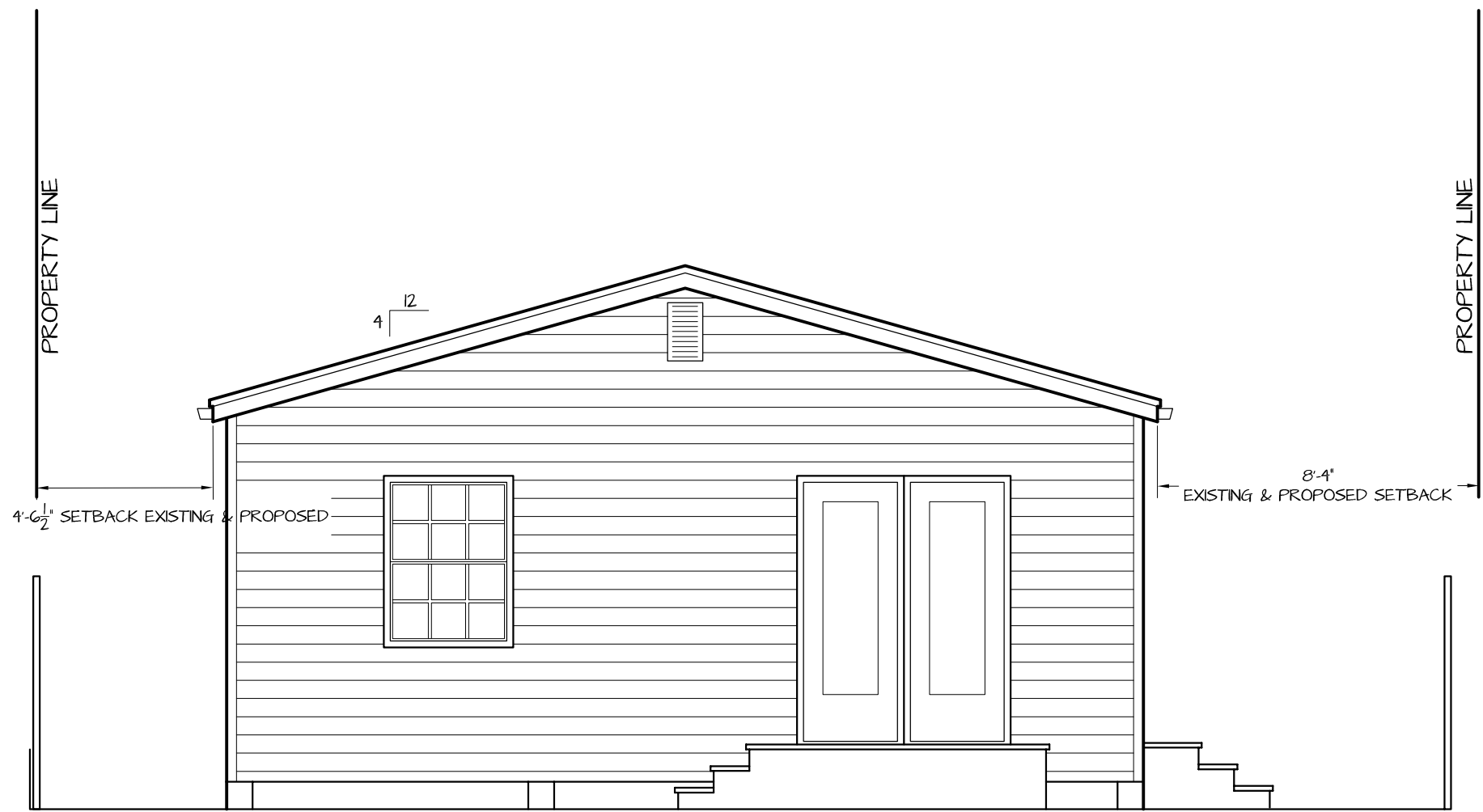
WEST ELEVATION 1/4" = 1'-0" EXISTING
