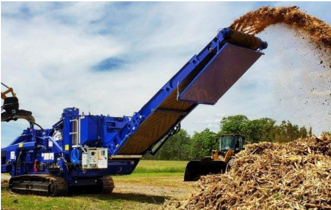
Visual reference: high-horsepower horizontal grinding capability for vegetative debris reduction.
