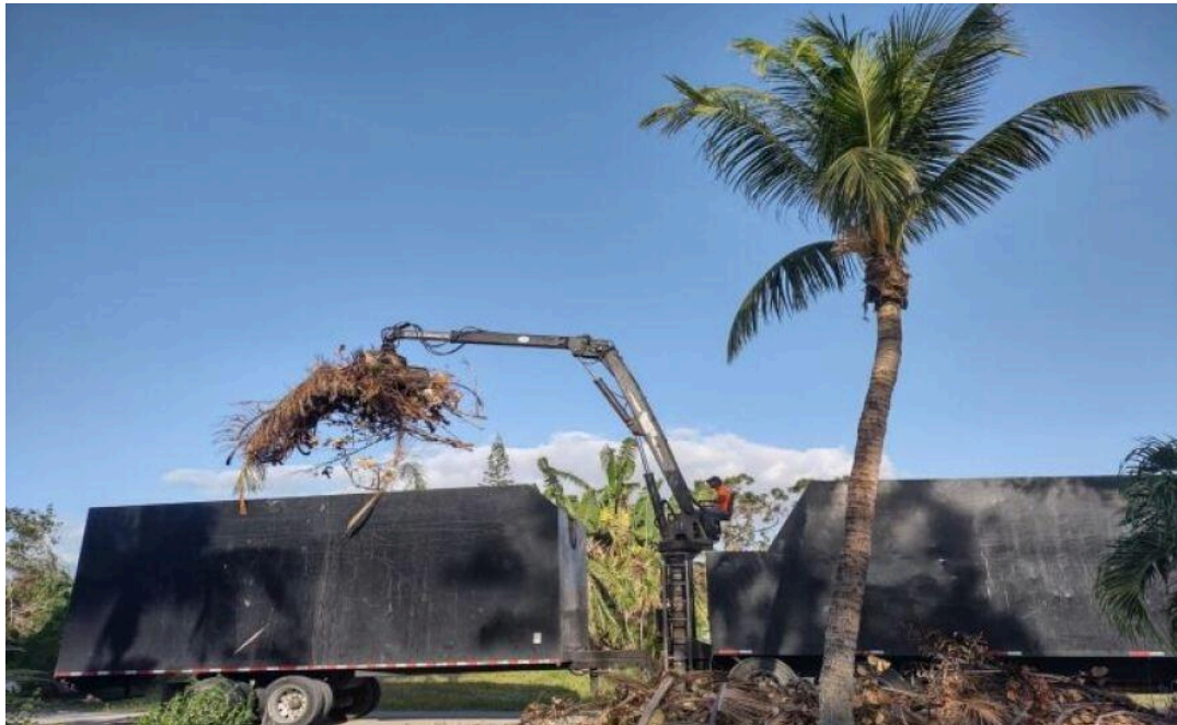
Visual reference: grapple truck loading vegetative debris for haul-out.
