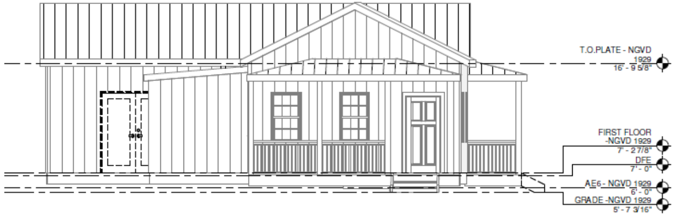
3 FRONT ELEVATION - DEMO/EXISTING A 4 1/4" = 1'-0"
