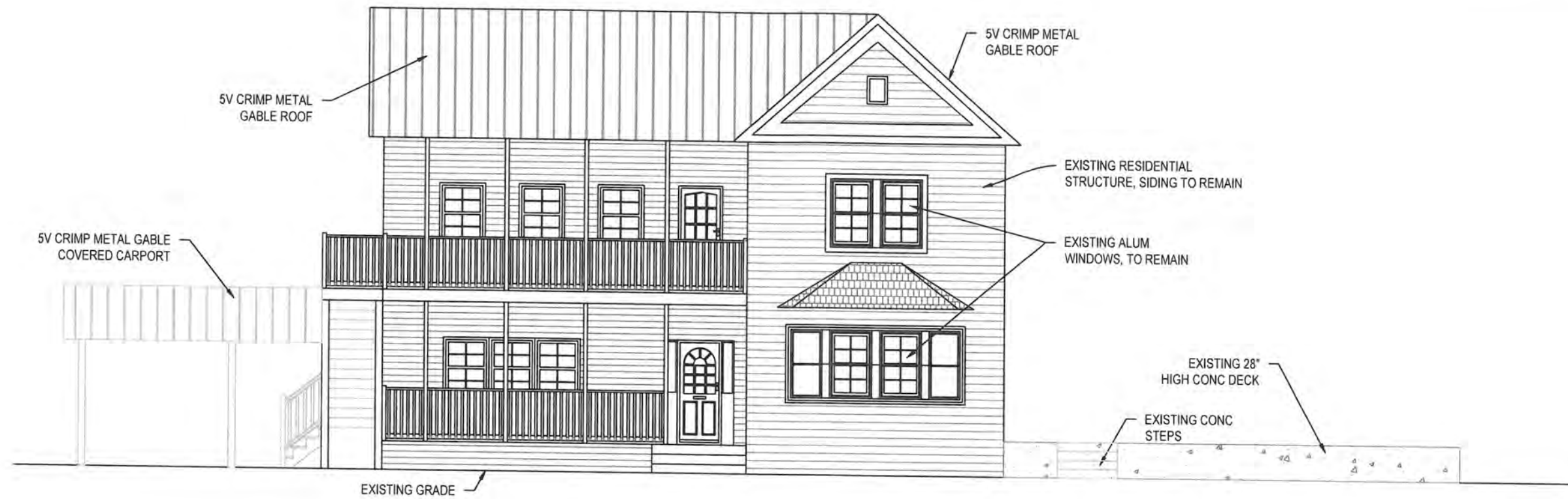
6 EXISTING ELEVATION VIEW - SOUTH S-2.0 SCALE: 1/8" = 1'-0"
