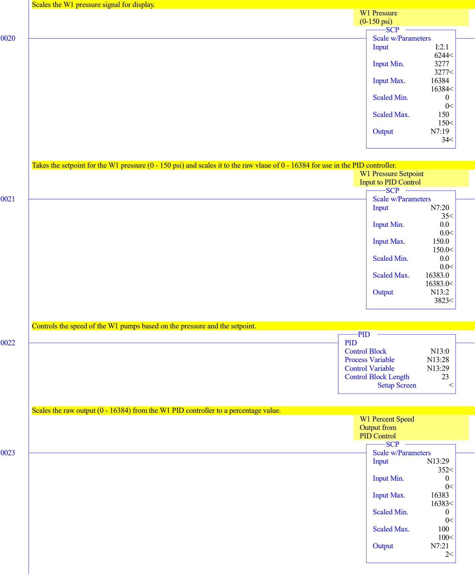
Scales the PID output to VFD frequency
