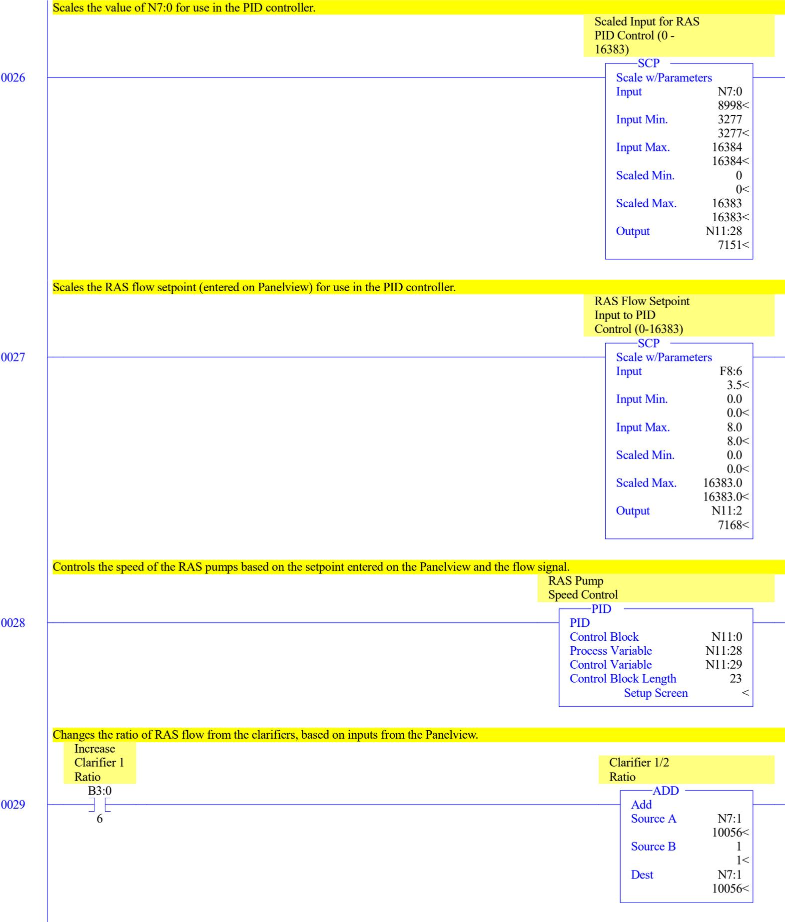
Changes the ratio of RAS flow from the clarifiers, based on inputs from the Panelview.
