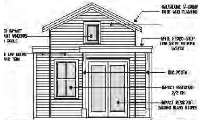
Front Elevation of Proposed Accessory Structure.
