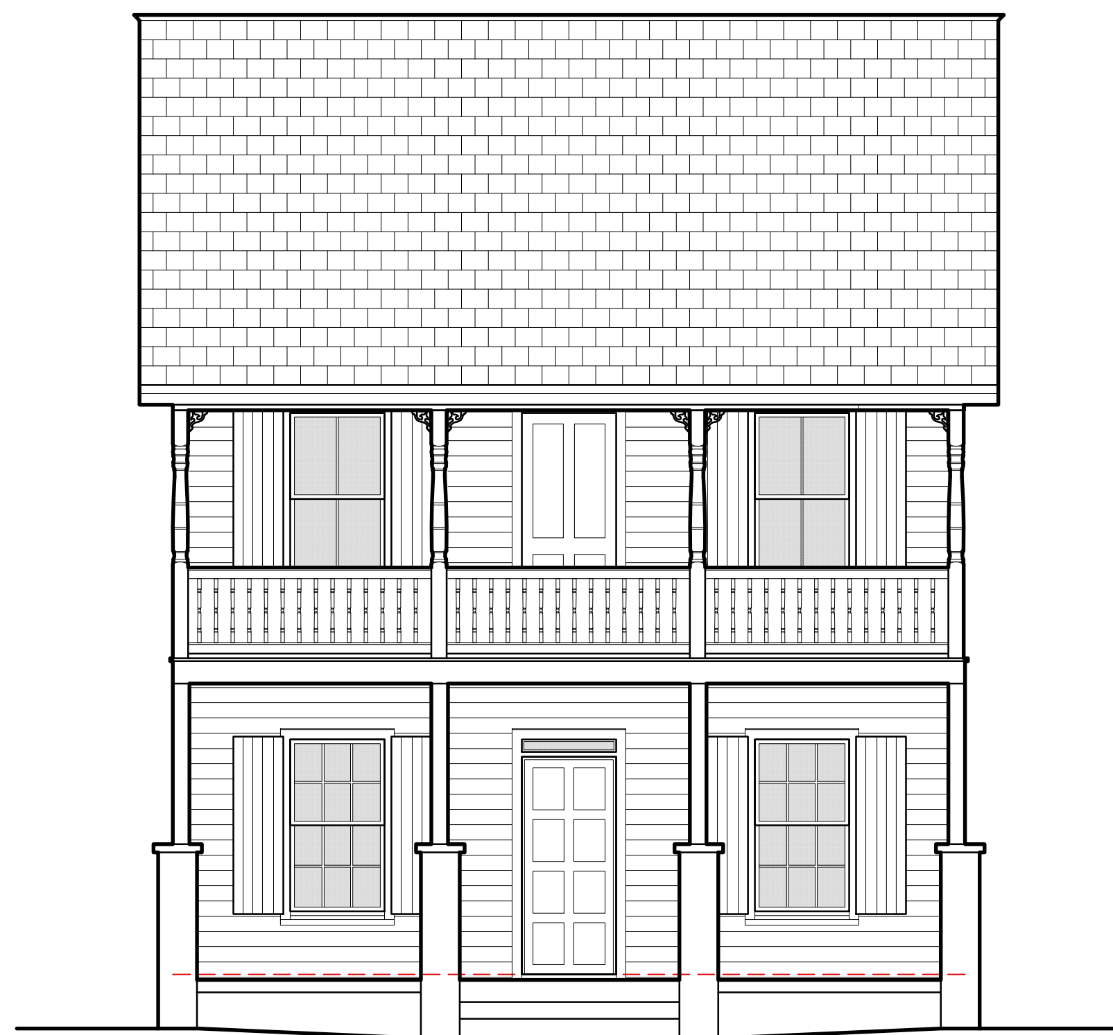
EXISTING FRONT ELEVATION 1/4"=1'-0"
