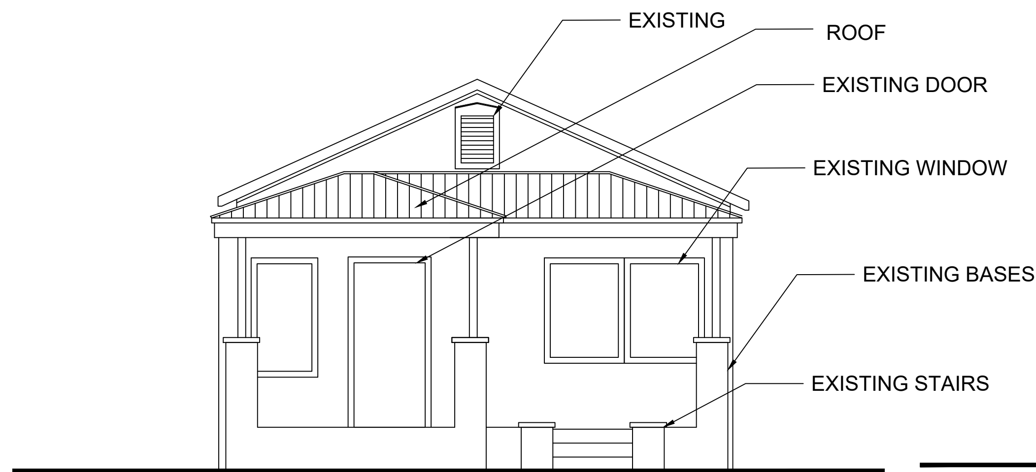
EXISTING FRONT ELEVATION 1/4" = 1'-0"
