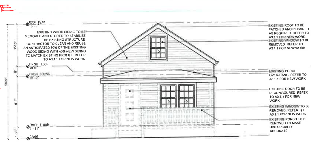
1 DEMOLITION SOUTH ELEVATION SCALE: 1/4"=1'-0"
