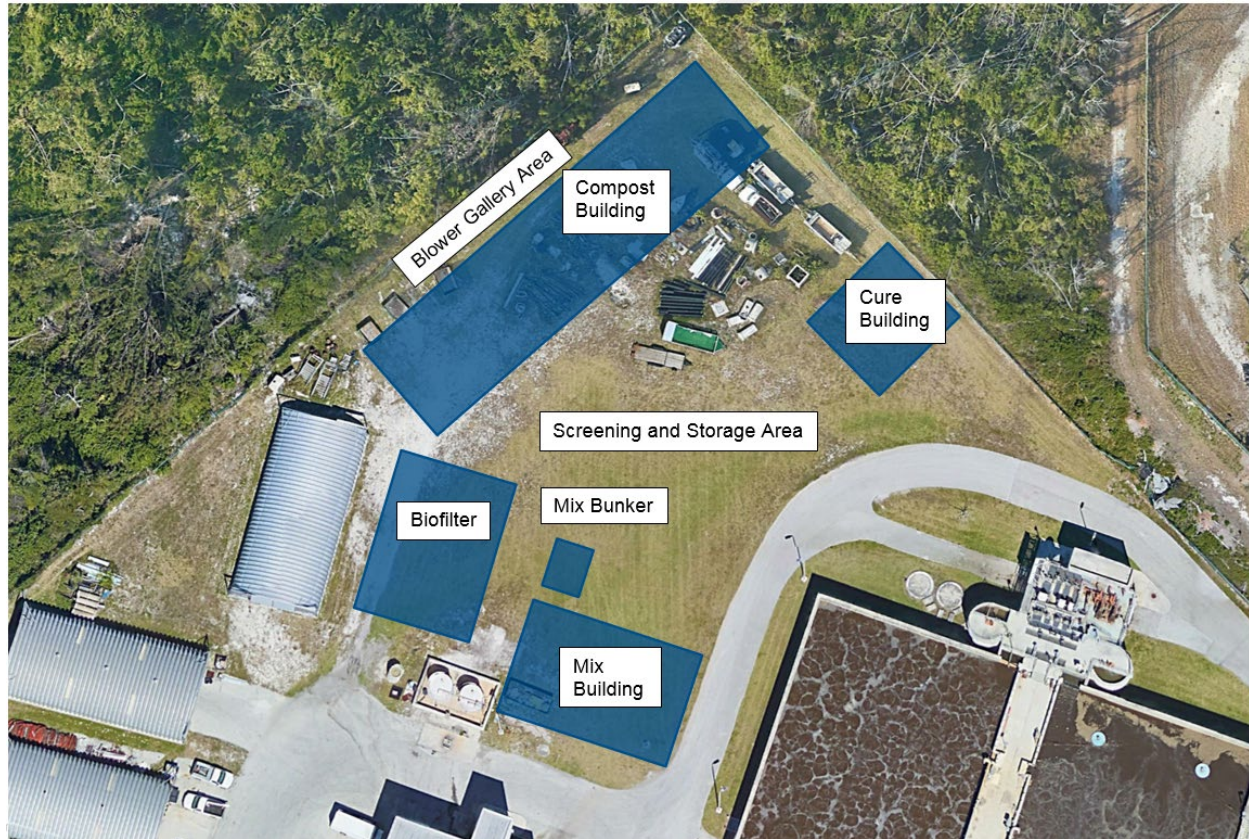
Figure 4. Concept Compost Site Layout with Major Facility Components (Scale is Approximate) Key West Biosolids Compost Facility Concept
