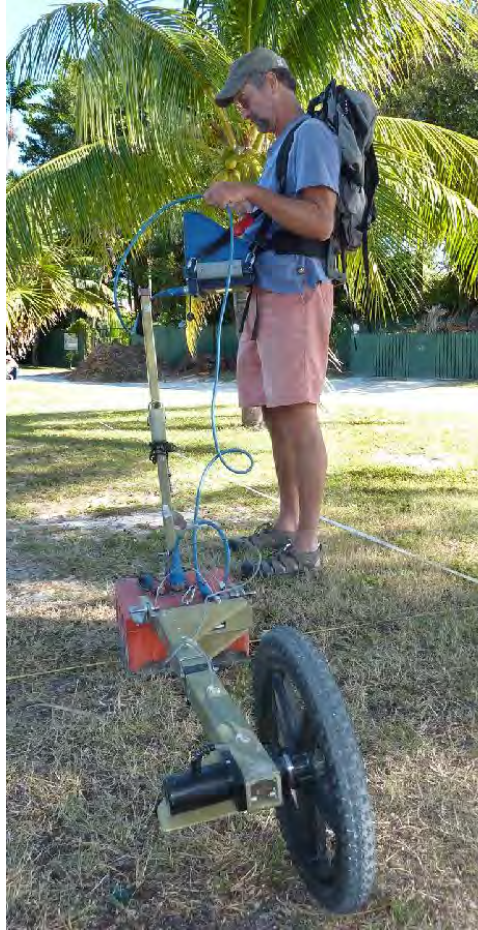
Figure 1: GPR system used in collection was the GSSI SIR-3000 system, 400 MHz antenna (orange box) and an attached survey wheel for distance calibration.
