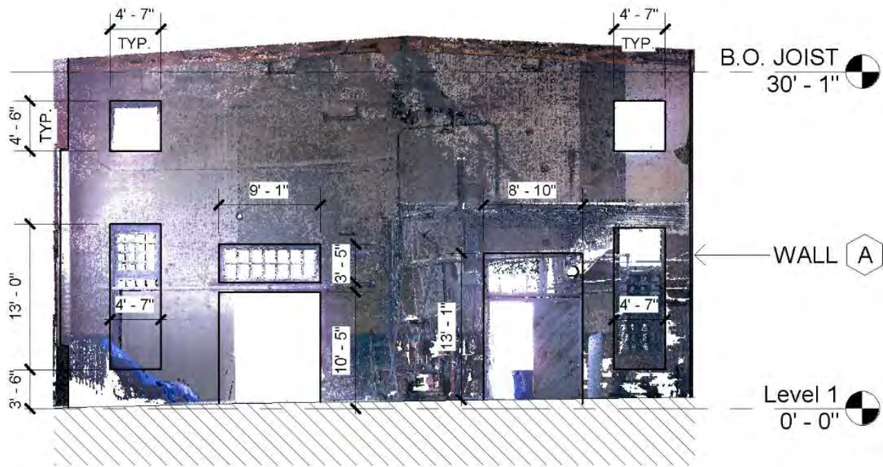
Figure A2: Building 1, Interior Wall A elevation from Point Cloud view.
