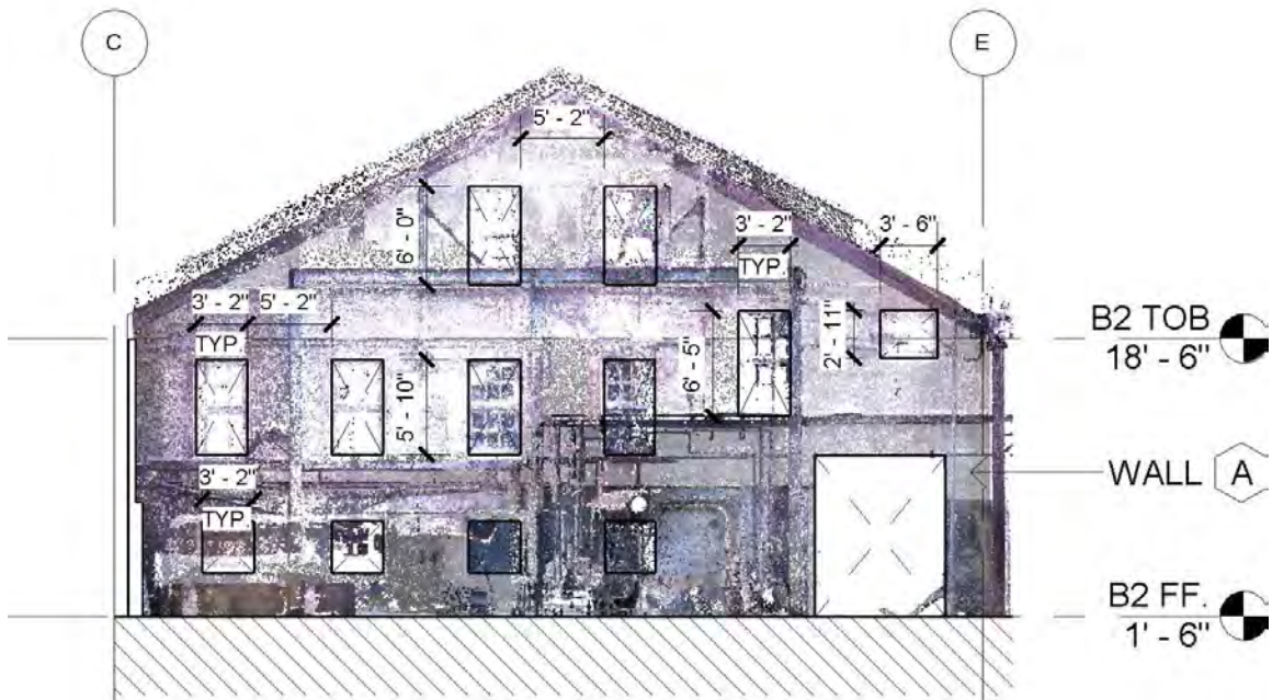
Figure B2: Building 2, Wall A from Point Cloud View.
