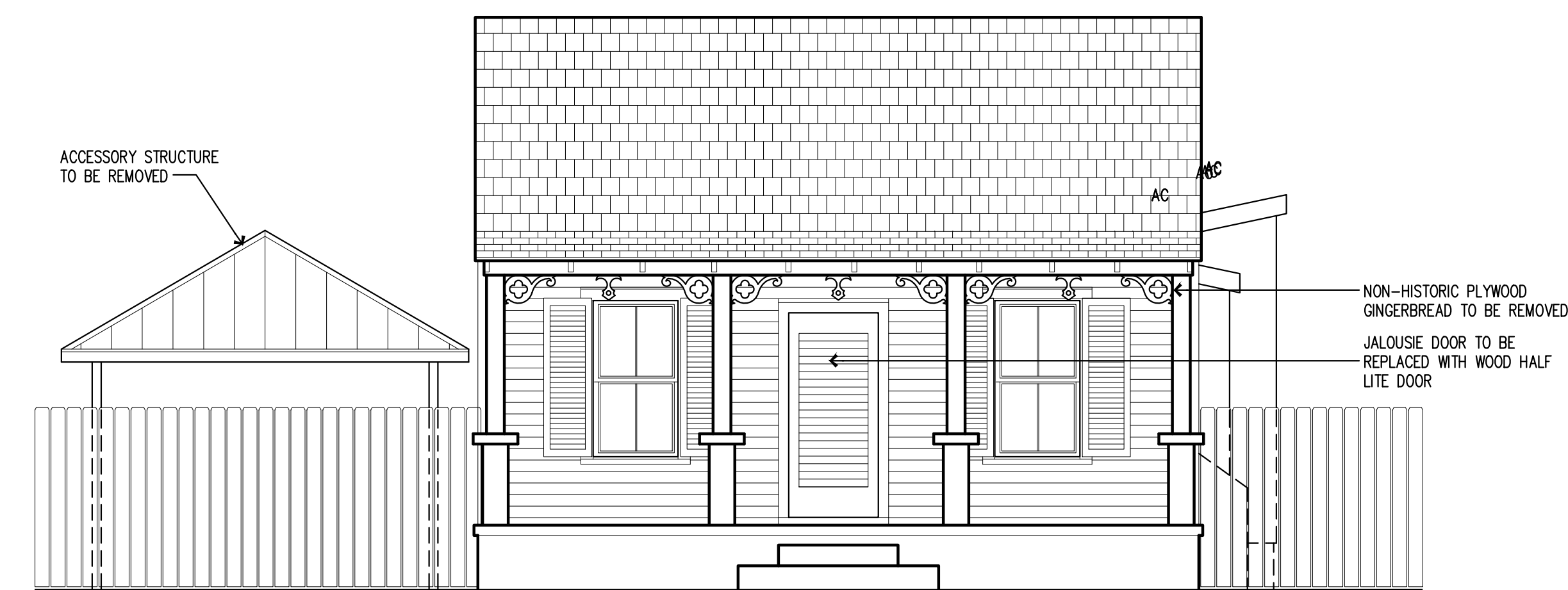
EXISTING FRONT ELEVATION 1/4"=1'-0" EXISTING
