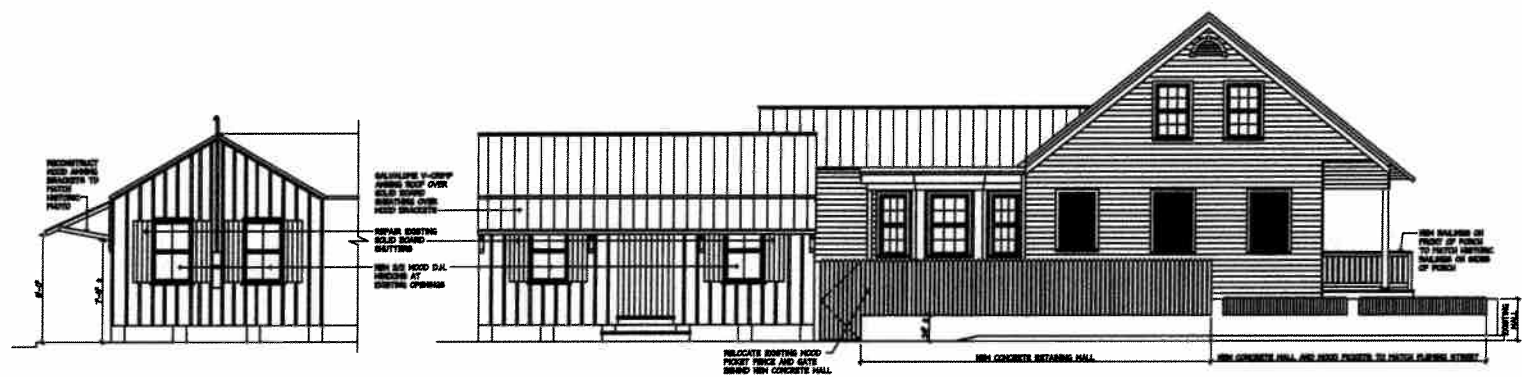
PROPOSED COTTAGE SIDE ELEVATION (NORTH) 1/4"=1'-0"
