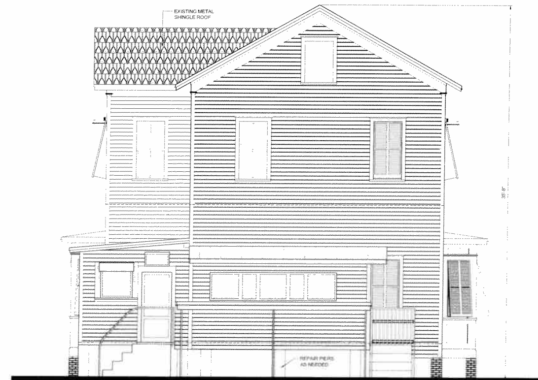
EXISTING SOUTHWEST ELEVATION
