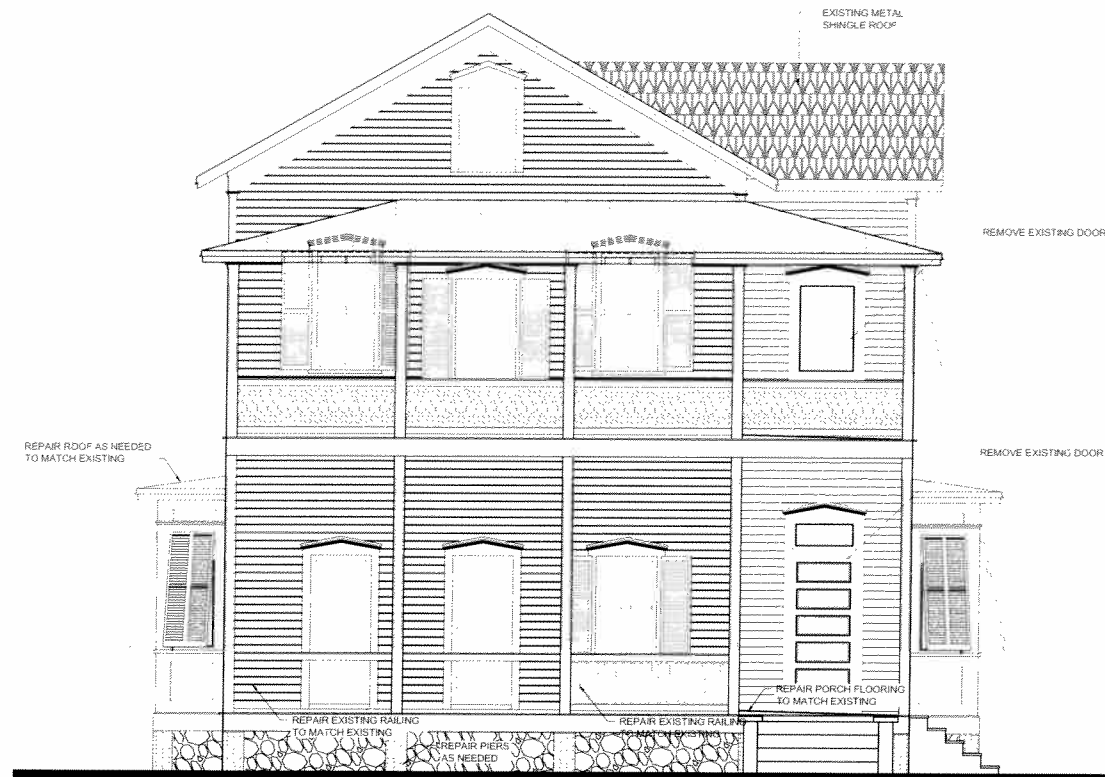
EXISTING NORTHEAST ELEVATION
