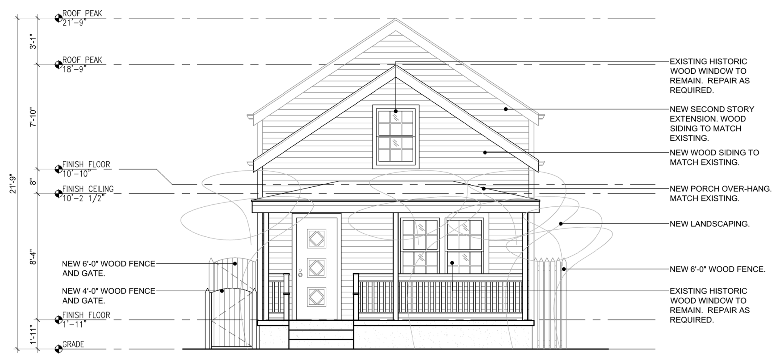
01 SOUTH/ FRONT ELEVATION A3.1.1 SCALE: 1/4" = 1'-0" GRAPHIC SCALE: 1/4" = 1'-0"
