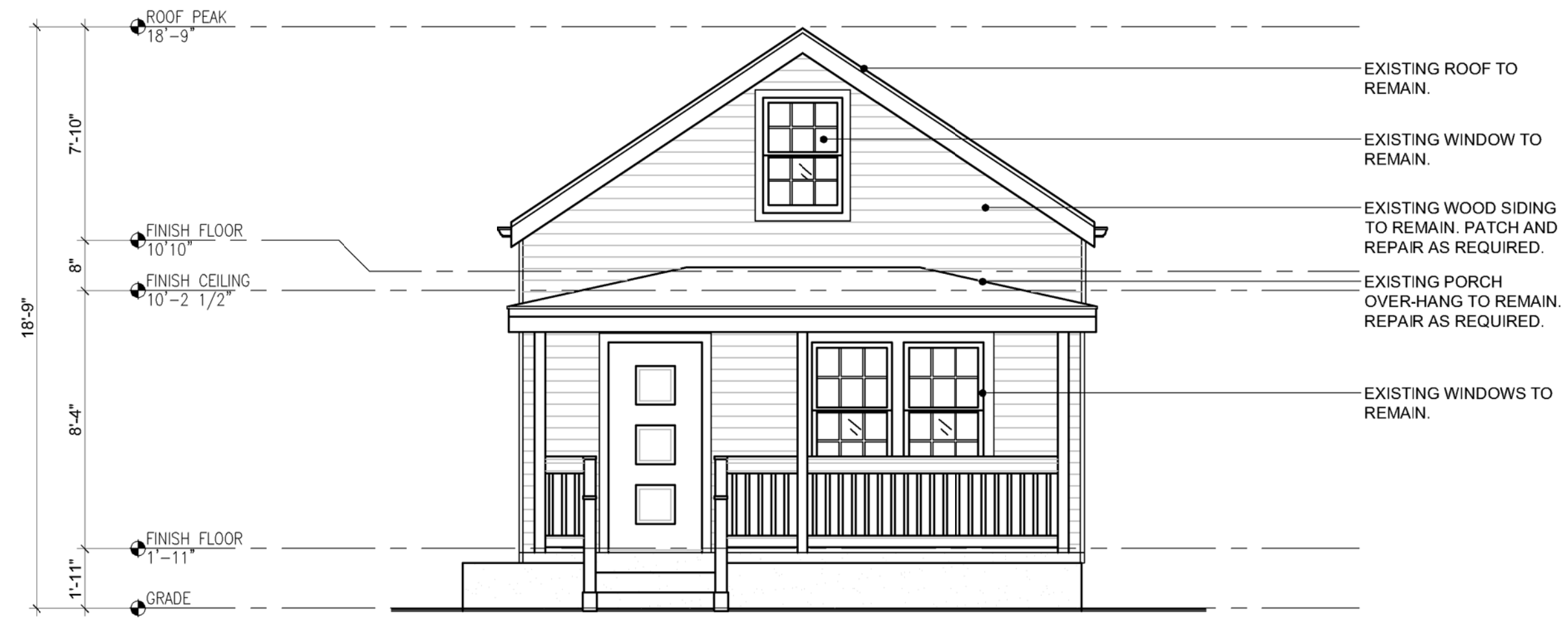
01 AE3.1.1 EXISTING FRONT ELEVATION SOUTH FACADE SCALE: 1/4" = 1'-0"
