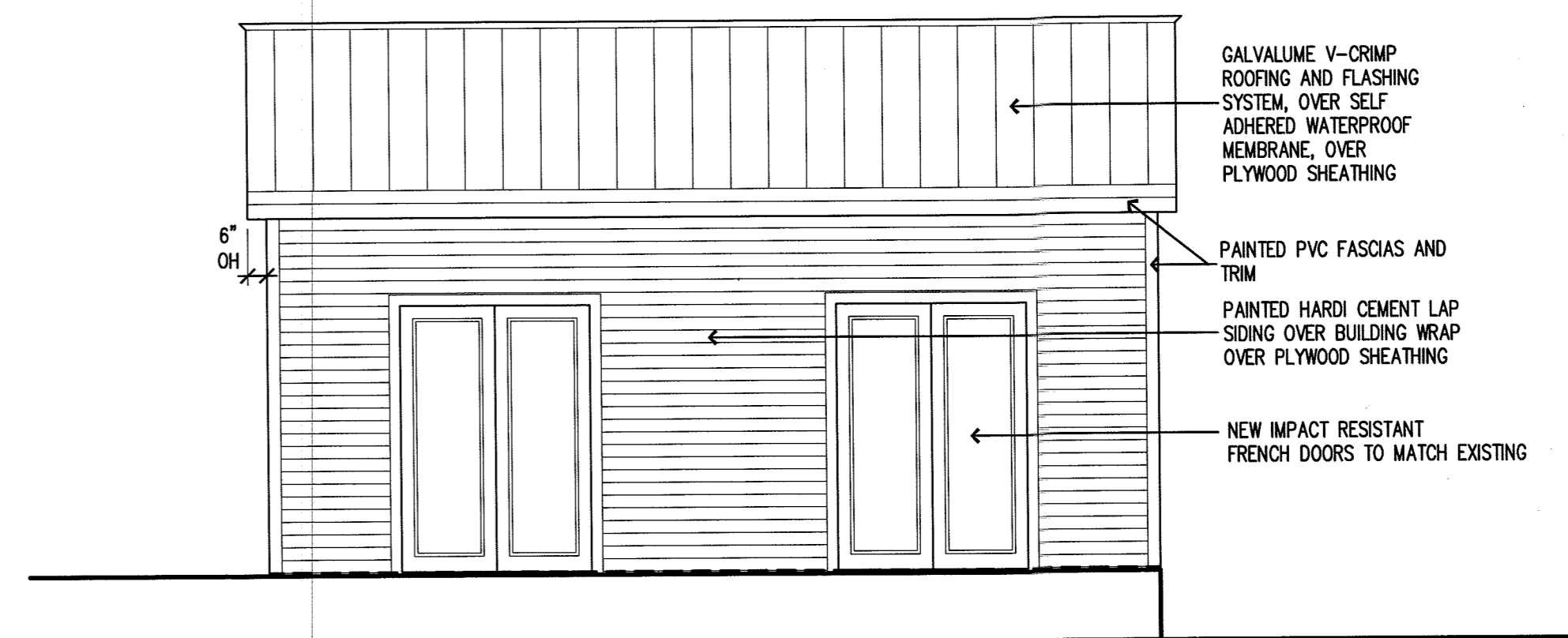
NEW NORTH ELEVATION 1/4" = 1'-0"
