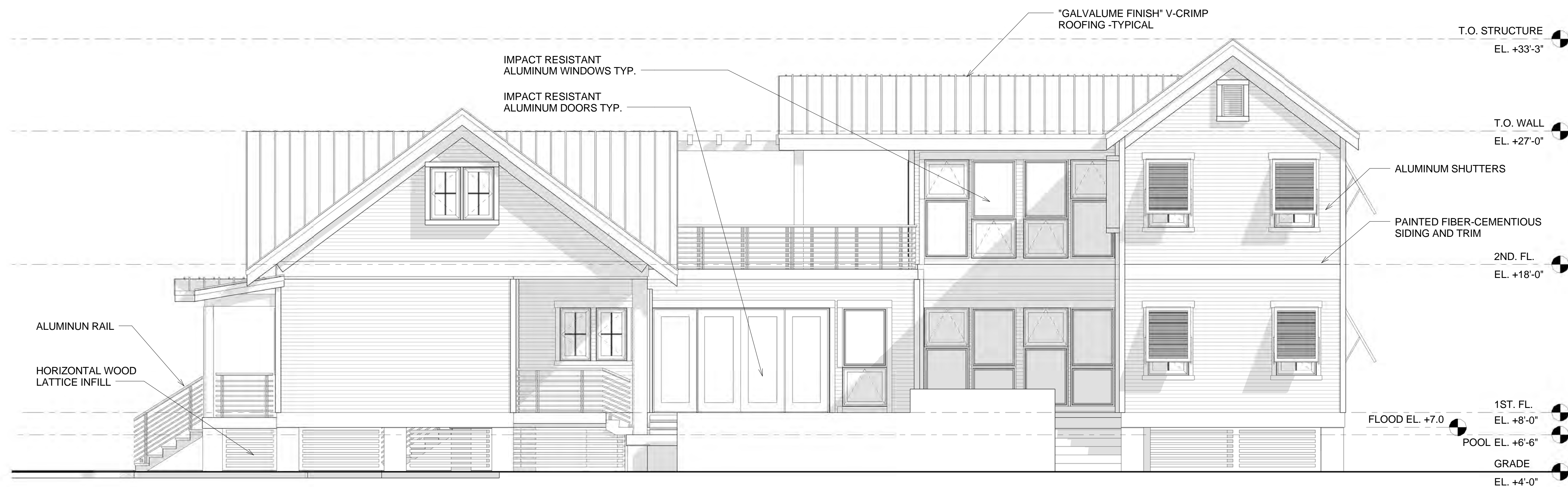
② NORTHEAST ELEVATION 1/4" = 1'-0"
